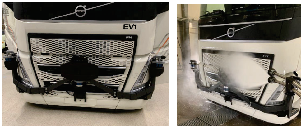
Figure 12 Testing on performance of sensor cleaning capacity as well as water intrusion
