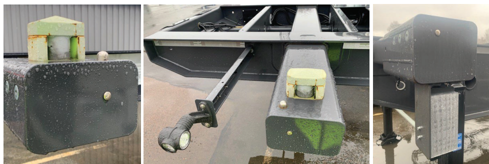
Figure 13 Automatic trailer locks with LED light indication
