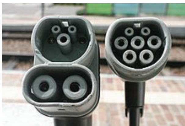
Figure 30 Connectors: Combo 2 (left), compared to IEC Type 2 (right). Two large direct current (DC) pins are added below, and the four-alternating current (AC) pins for neutral and three-phase are removed.
