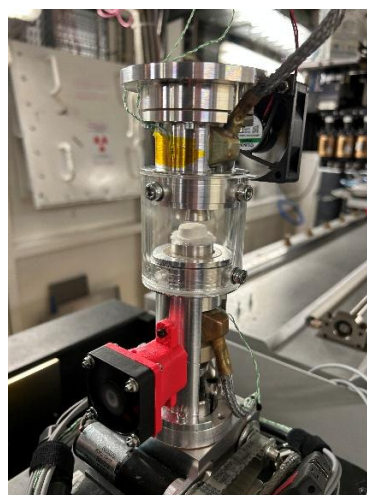
Figure. Fiber pad after compression into a 3D shape using the LTH in-situ compression cell.
