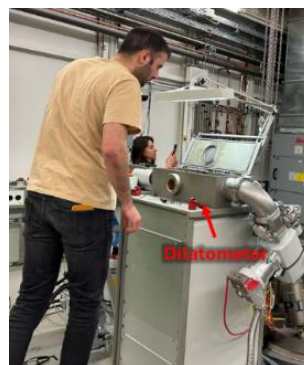
The dilatometer used for in-situ SAXS/WAXS experiments at P07
