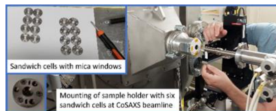
Figure 1. Sandwich cells (left) and the experiment setup at CoSAXS beamline (right).
