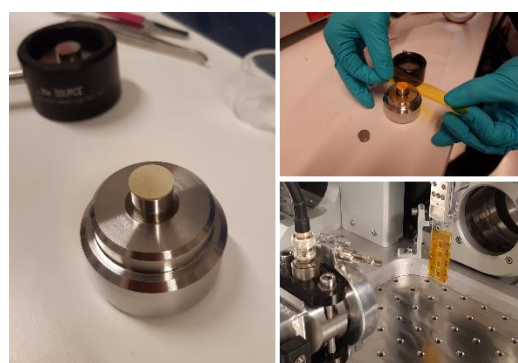
Figure 1 Arevo's biostimulants were milled to a fine powder and then pressed to a disk for mounting at the Balder beamline at MAX IV Laboratory.
