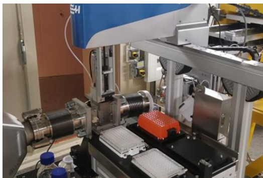
Figure 1: High-throughput SAXS setup at CoSAXS, with autosampler and flow cell.
