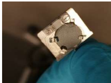
Figure 1. A circular coated electrode mounted in a sample holder, ready for SR-XPS at MAX IV.
