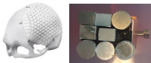
Figure 1. a) OssDsigns cranial implant. b) AM samples (circular) and PE reference samples (square) immersed in DPBS.
