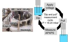
The sample holder has slots for the sample, which also acts as working electrode, as well as for the SCE reference- and Pt counter electrodes. The sample holder was placed on the manipulator in the vacuum chamber
