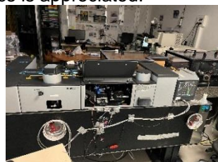
Figure 1. sSNOM instrument (Nano IR) at the SMIS 1 beamline at Soleil.
