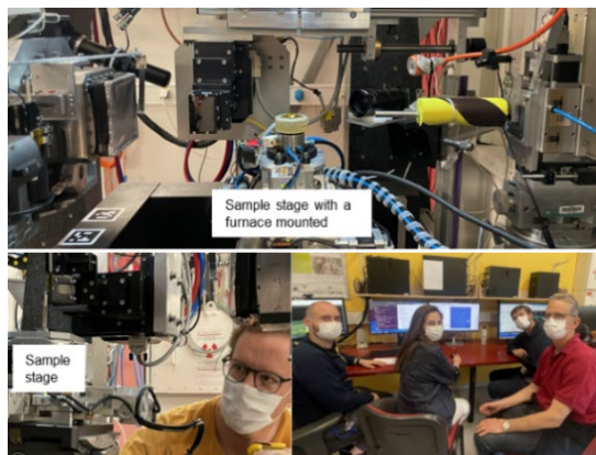
Figure 1. top: 3DXRD setup with a furnace on sample stage, bottom left: Adjustment of the sample setup for DCT measurement and bottom right: and controlling and following the experiment together with ESRF instrument scientists.
