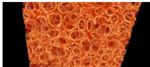
Figure 2. Visualisation of PUR cell structure.
