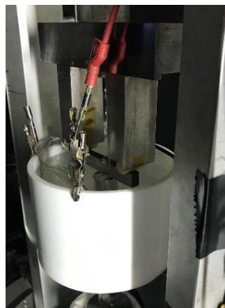
Experiment setup at NeXT. Specimen is under mechanical load during electrochemical charging before neutron imaging.
