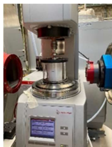
Figure 1. Rheo-SANS experiment with a white paint under shear in the central upright standing cylinder. The neutron beam comes from the right side through the red and blue colored apparatus and continues through the sample. Scattered neutrons pass the left circular window before detection by a 2D detector.
