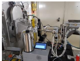
Figure Linkam capillary temperature cell at CoSAXS, MAX IV.
