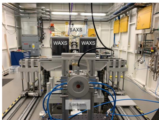
Figure 1. Experimental set-up at P21 with the water-cooled and Ar-protected furnace in the foreground.
