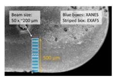
The EXAFS measurements on selected regions of the worn areas also showed changes in bond distances and number of neighbours between the atoms of the coatings compared to the corresponding asdeposited reference coatings. Additional TEM investigations revealed formation of nm-sized domains enriched in TiN.
