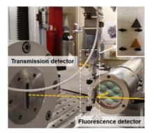
The chemical changes across the surface of the tool were probed by measurements at the Ti K absorption edge. Additional measurements at the Cr-K and Fe-K edges were made to investigate the nature of the steel species adhered to the tool. Complementary studies of structural changes were performed by transmission electron microscopy (TEM) at Linköping Uni.
