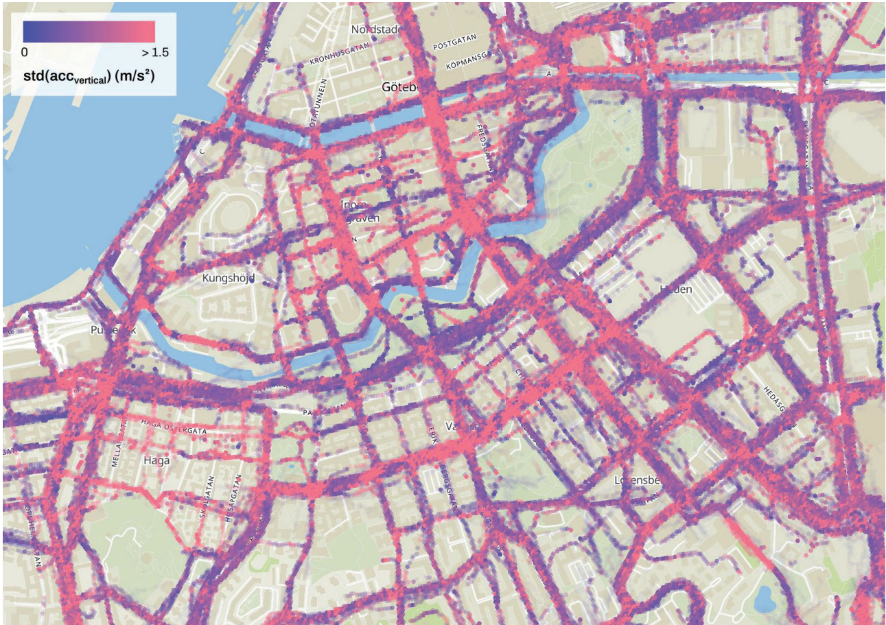
Figure 19: Overview of the estimated road roughness in Gothenburg. Yellow represents smoother surfaces; red represents rougher surfaces.
