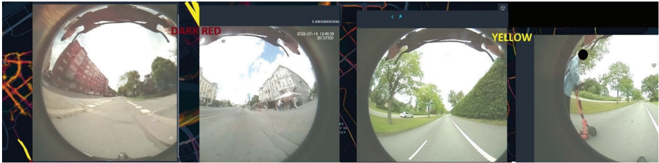
Figure 18: Examples of two different segments identified as rough (dark red) vs two segments identified as smooth (yellow).
