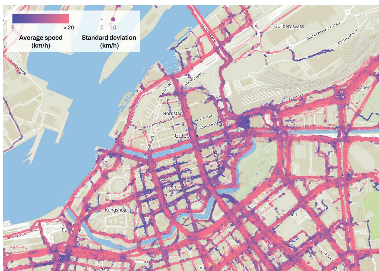
Figure 22: Observed average (blue: low value, pink: high value) and standard deviation (low: small circle radius, high: large radius) for each speed distribution for each H3-node.
