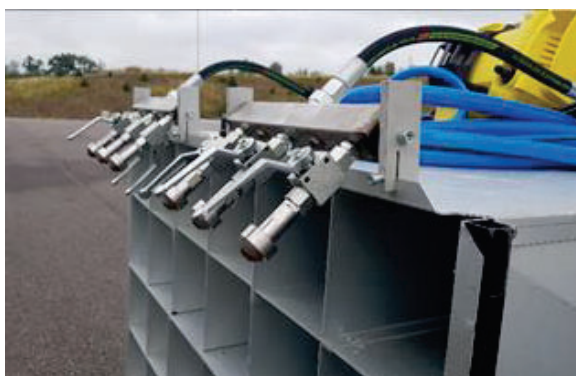
Figure 7 Spray nozzles on spray rig v1
