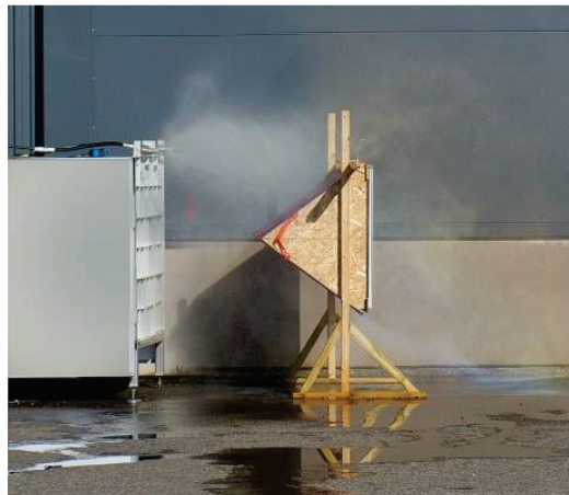
Figure 28 Spray rig v1 with target in front
