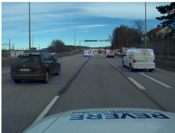
Figure 12: Example of medium and urgent warning are demonstrated in this image. The example traffic safety KPI “collwarn” depends on the relative speed and reachability of the target vehicle in relation to the ego vehicle.
