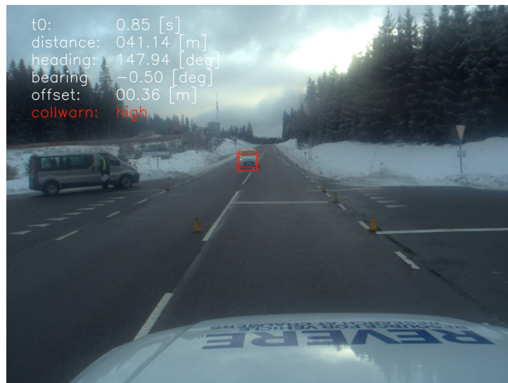
Figure 6: Annotated collision scenario with urgent collision warning, actions need to be taken.
