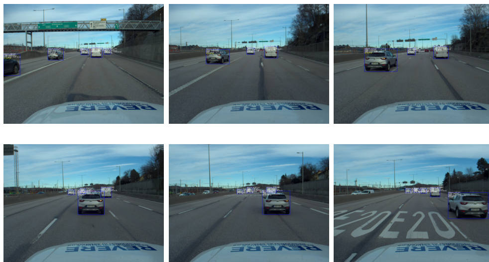
Figure 14: A sequence of a target vehicle performing a lane change in front of the ego vehicle. The sequence of images are annotated with the heading and relative velocity to the ego vehicle. The “collwarn” signal (described in Sec. 6.3.2) is indicated in the annotations.
