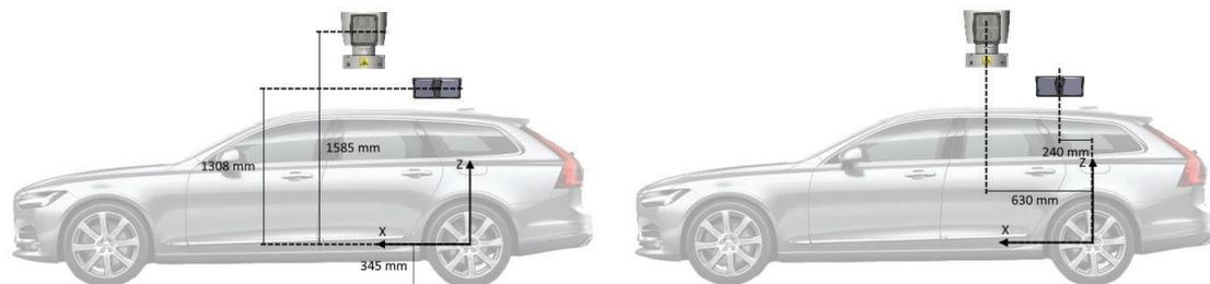
Figure 18 The mounting locations of the side looking lidars relative to the center of the rear axle. Offsets in Z are seen on the left and offsets in X are seen on the right.
