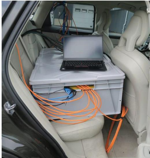
Figure 23 The figure shows box with battery power supply, fuses, converters, switches and a computer for logging that is accessed via a laptop. Orange cables are for Ethernet. Blue cables are for serial communication to the radars.
