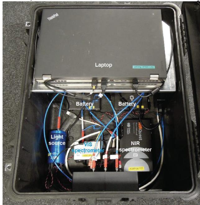
Figure 9. The assembled portable spectral reflectance measurement device. Blue cables are optical fibers connected to the spectrometers and light source. These are accessible from outside the box via a panel in the lower part of the image.
