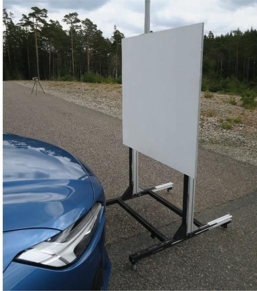
Figure 10 The 50% Permaflect target used in the linear calibration method, mounted on a target carrier.
