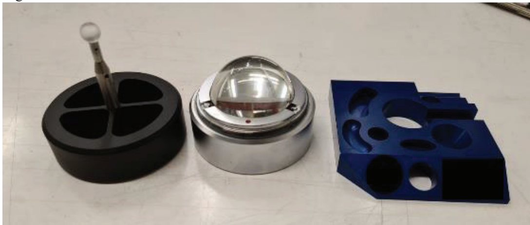
Figure 3: Objects that illustrate increased complexity in determining the centre of the object. Glass sphere used for daily control of a coordinate measuring machine (left). Glass hemisphere used to as a reference in roundness measurements (middle). Coordinate measuring machine evaluation gauge (right).
