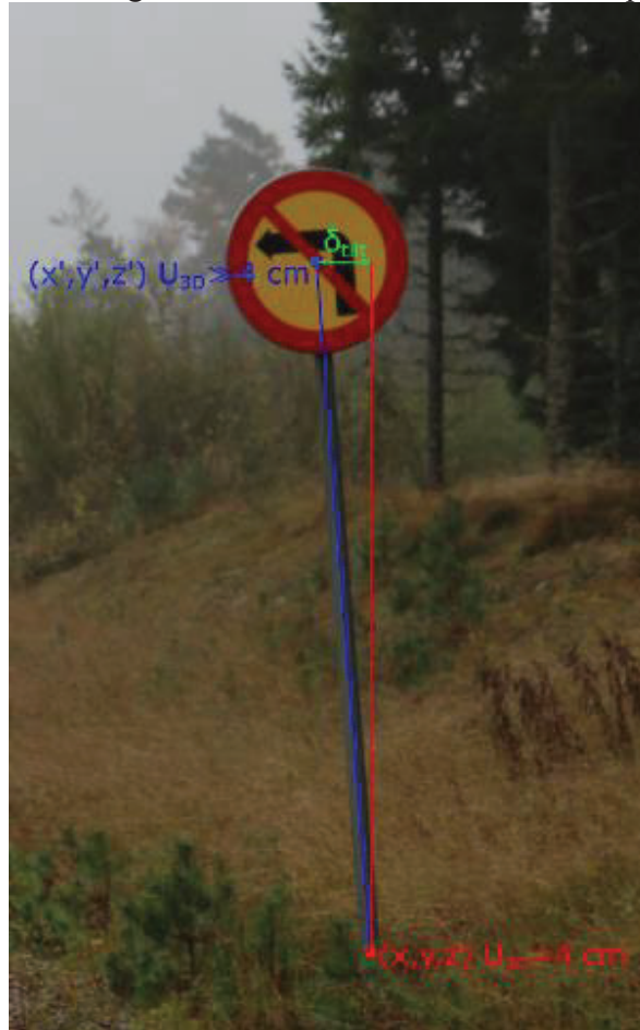
Figure 4: Illustration of how an expanded 3D measurement uncertainty valid for the bottom of the pole can't be used as a reference value for the centre of the sign due to other uncertainty contributions such as the tilt of the sign.
