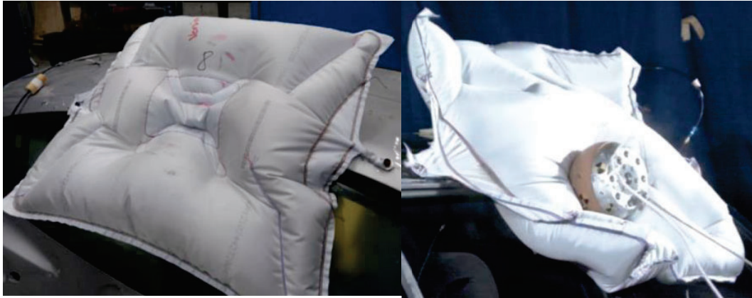
Figure 13a: Image of the inflated external airbag on top of the B-pillar, covering the roof edge.
