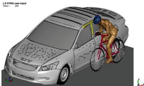
Figure 12a: Simulation of expandable B-pillar concept in LS-Dyna.
