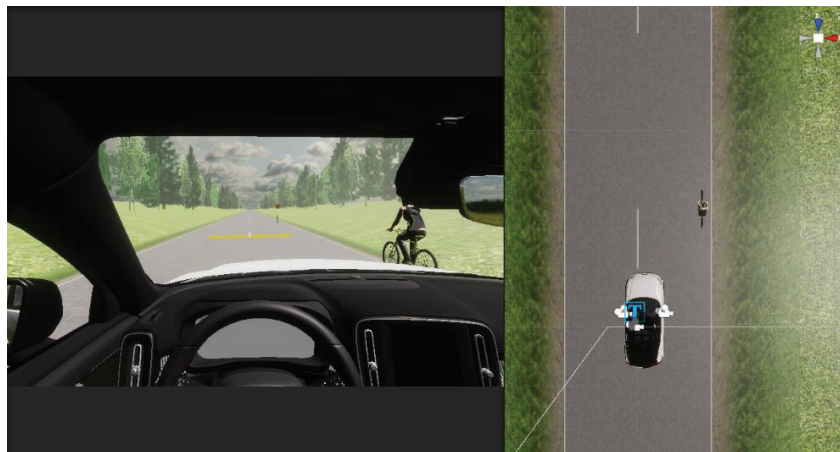
Figure 33: Yellow bar indicates - when lateral clearance is between 1.5 to 0.5m to the cyclist.
