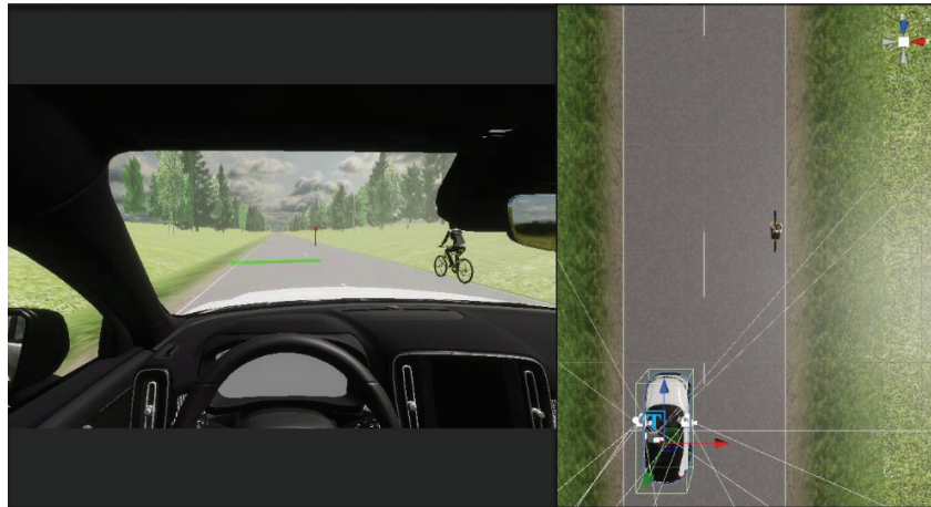
Figure 32: Green bar indicates - when lateral clearance is greater than 1.5m to the cyclist.
