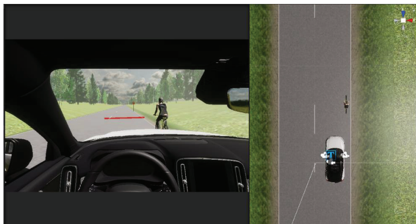
Figure 34: Red bar indicates - when lateral clearance is less than 0.5m to the cyclist.
