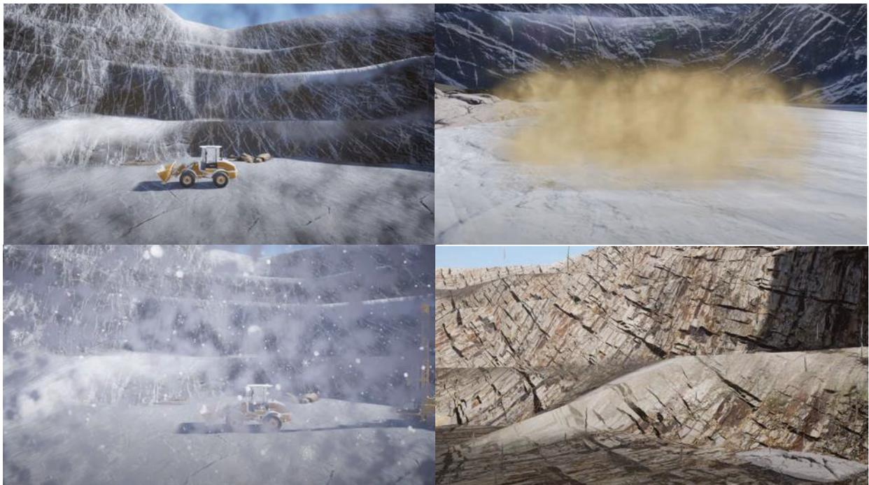
Figure 1. The Carla Simulator has been extended to be able to generate data with dirt on the sensor, dust clouds as well as snow.
