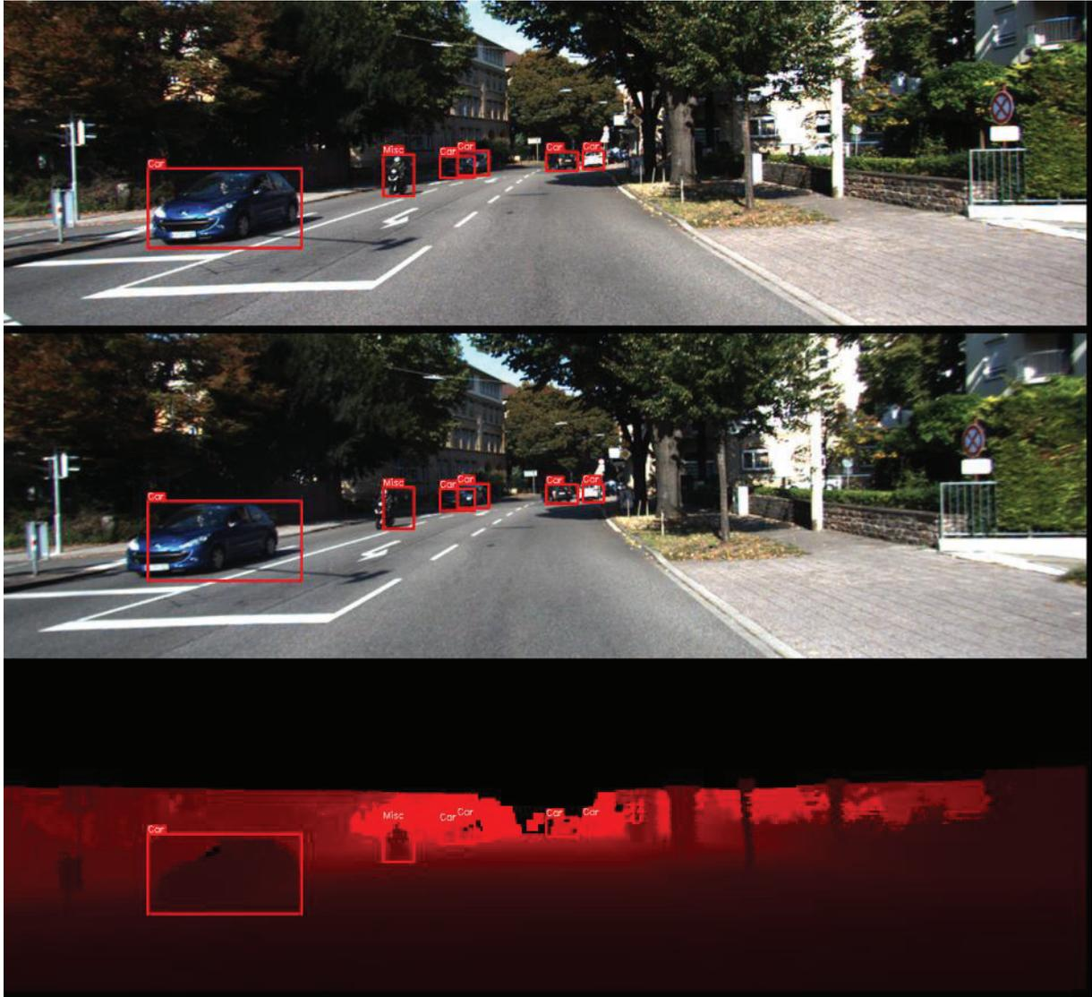
Figure 13. Example of an annotated sample from the dataset: the mono/left stereo image (top), the right stereo image (center), and the depth image (bottom).
