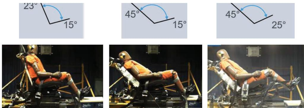
Figure 7. Schematics and photos of test with crash test dummies showing the three seating positions used in the tests. Left: seatback angle upright, middle: seatback angle reclined, right: seat pan angle raised.
