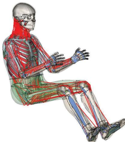
Figure 4. The SAFER HBM v10.0 with soft tissues made transparent to show the skeletal structure and muscle elements.
