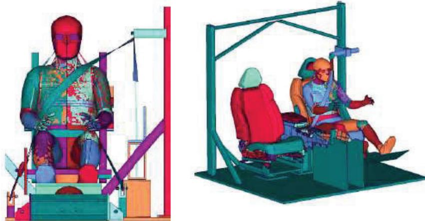
Figure 5. The SAFER HBM v10.0 Far-Side impact validation study based on Pipkorn et al. (2021). Left: generic lab environment Far-Side test setup. Right: Vehicle-based Far-Side test setup.
