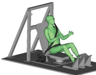
c) 'Pelvis seatbelt loading'      d) 'Sled test with rigid seat'
