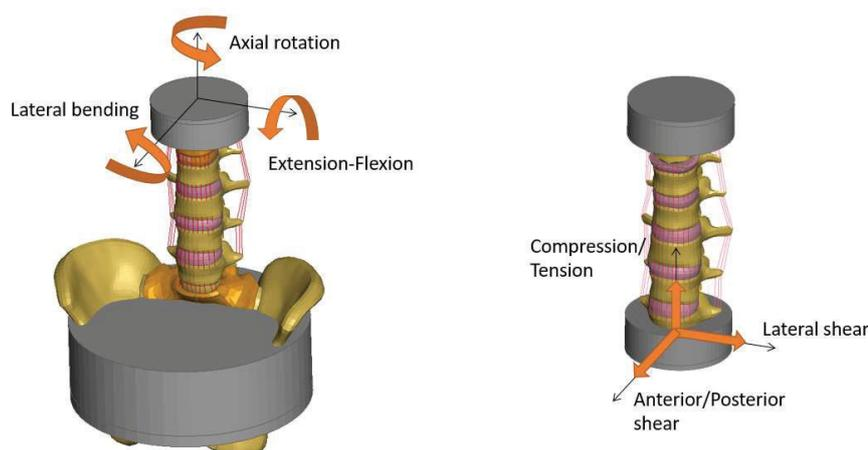
Figure 2. Illustration of the validation setups for the lumbar spine validation. Left: Yamamoto et al. (1989). Right: Demetropoulos et al. (1998). The orange arrows show the directions of the displacements applied.
