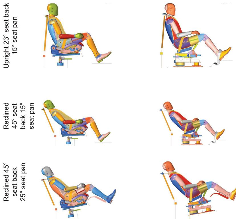
Figure 10. The THOR model in the production seat and the semi-rigid seat models
