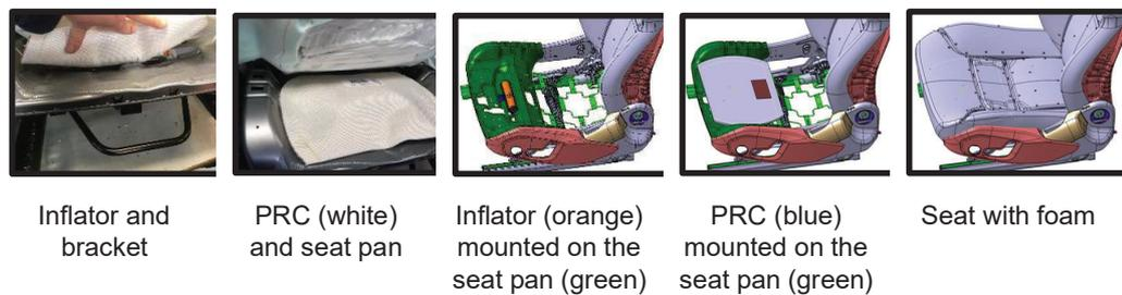
Figure 8. Photos and finite element models of the pelvis restraint cushion
