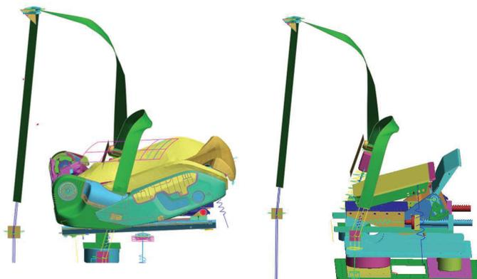
Figure 9. The models of the production seat (left) and the semi-rigid seat (right)
