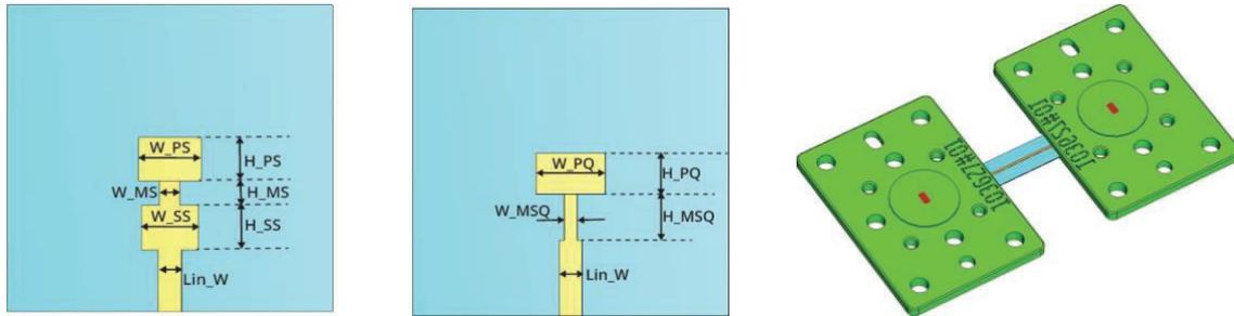
Figure 17. different matching techniques of the transition operating at 140 GHz
