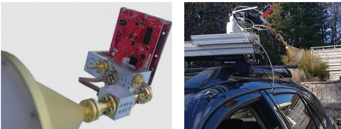
*Figure 20 The 77-81 GHz polarimetric radar.*
