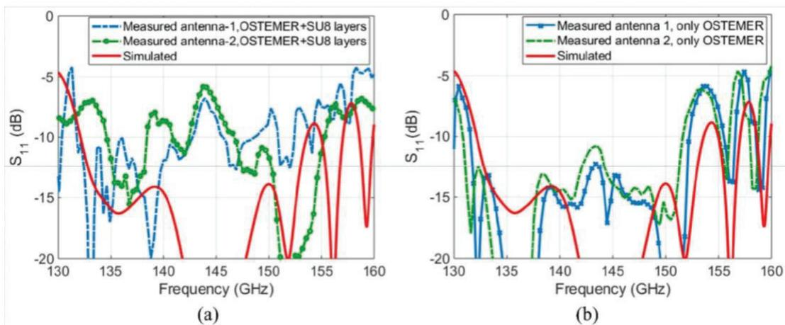
Figure 9: Simulated and measured  $S_{11}$  for the  $16 \times 16$  element antenna array. (a) The slot layer was made of SU8, the cavity layer, and the feed layer was made of OSTEMER, (b) all layers were made of OSTEMER.
