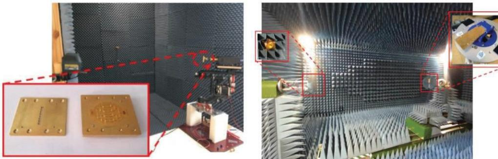
Figure 3 far-field measurement setup at Chalmers and Gapwaves .
