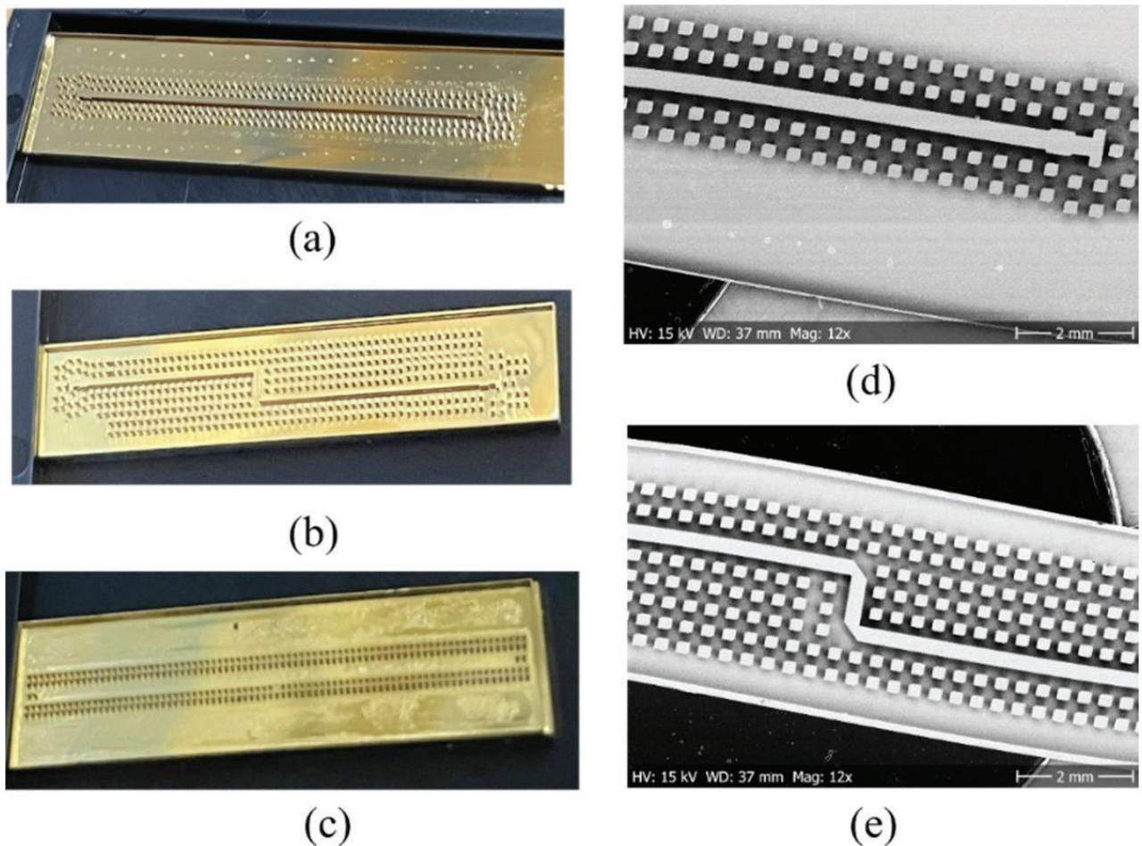
Figure 12: Fabricated chips: (a) straight RGW on chip (b) bent RGW chip, (c) groove GW chip. SEM images of the fabricated chips: (d) straight RGW, (e) bent RGW
