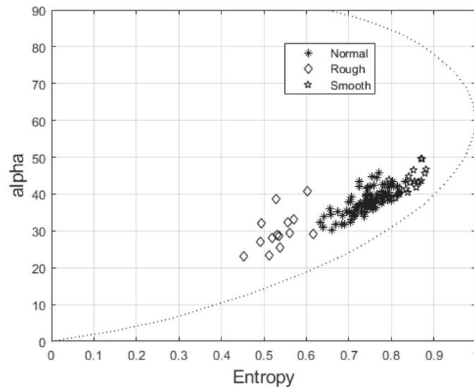
Figure 23  $\alpha$ , entropy plot for dry surfaces of different roughness. Normal: this is a surface with roughness, which is typical for the majority of public roads. We assume surface, RMS value  $\approx 0.9\text{mm}$ . Rough: we do not know the value of roughness for this surface but we assume RMS of 3-6 mm. Smooth, that would be typical for new asphalt surface.
