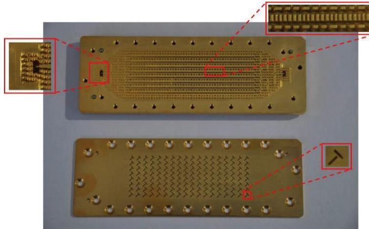
Figure 2 prototype of the dual circular polarized antenna 2. [2]
