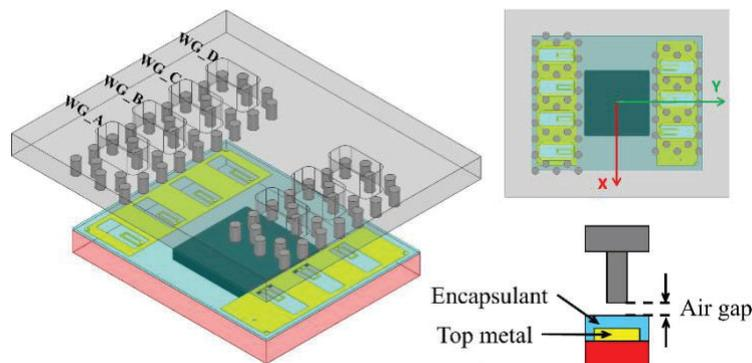
Figure 16. Compact gap waveguide interconnects for the LiP transceivers
