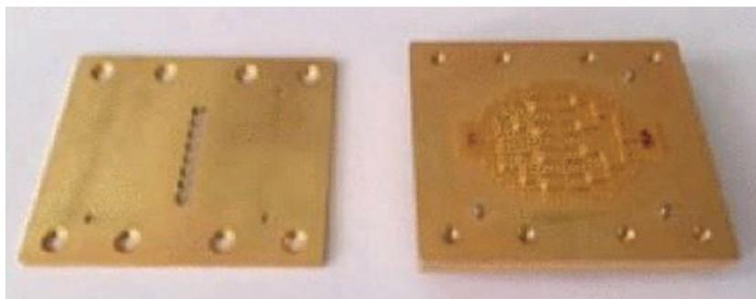
*Figure 1 prototype of the dual circular polarized antenna 1. [1]*
