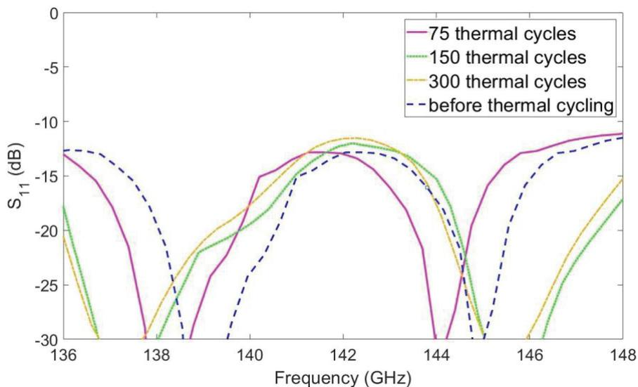
Figure 11: Simulated and measured  $S_{11}$  of the fabricated antenna before and after thermal cycling test.
