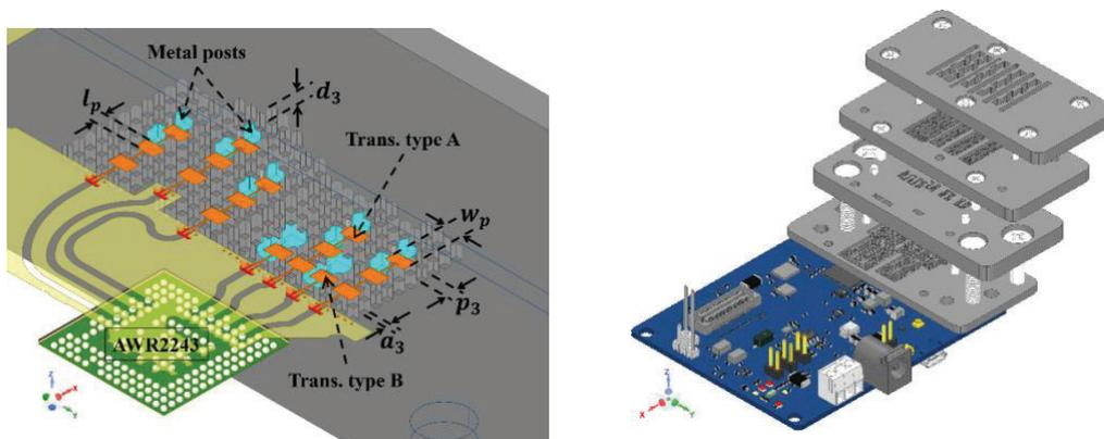
Figure 17. microstrip to waveguide transitions for the integration of radar transceivers with gap waveguide antenna.
