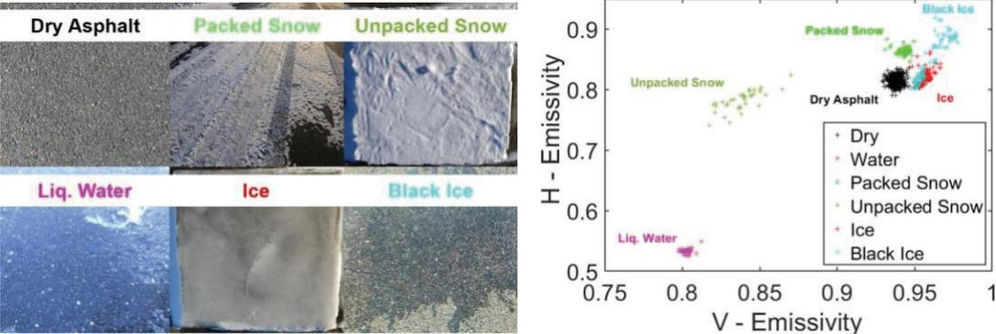
Figure 19 Six types of surfaces characterized by their emissivity for H and V polarizations
