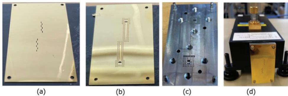
Figure 10: The fabricated antenna, (a) slot layer, (b) feed layer, (c) supporting bottom plate with WR-6.5 opening and gap waveguide pin flange structure, (d) fabricated antenna mounted in the machined supporting plate and connected to the VDI D-band extender.
