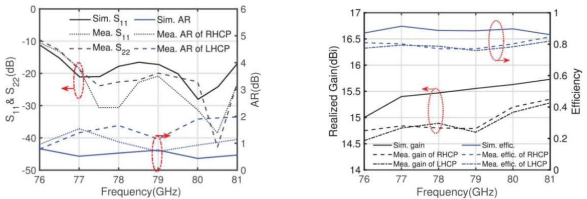
Figure 4 Measurements results of the dual circular polarized antenna 1.
