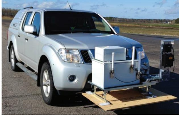
Figure 27 Radar setup to carry out dynamic measurement.
