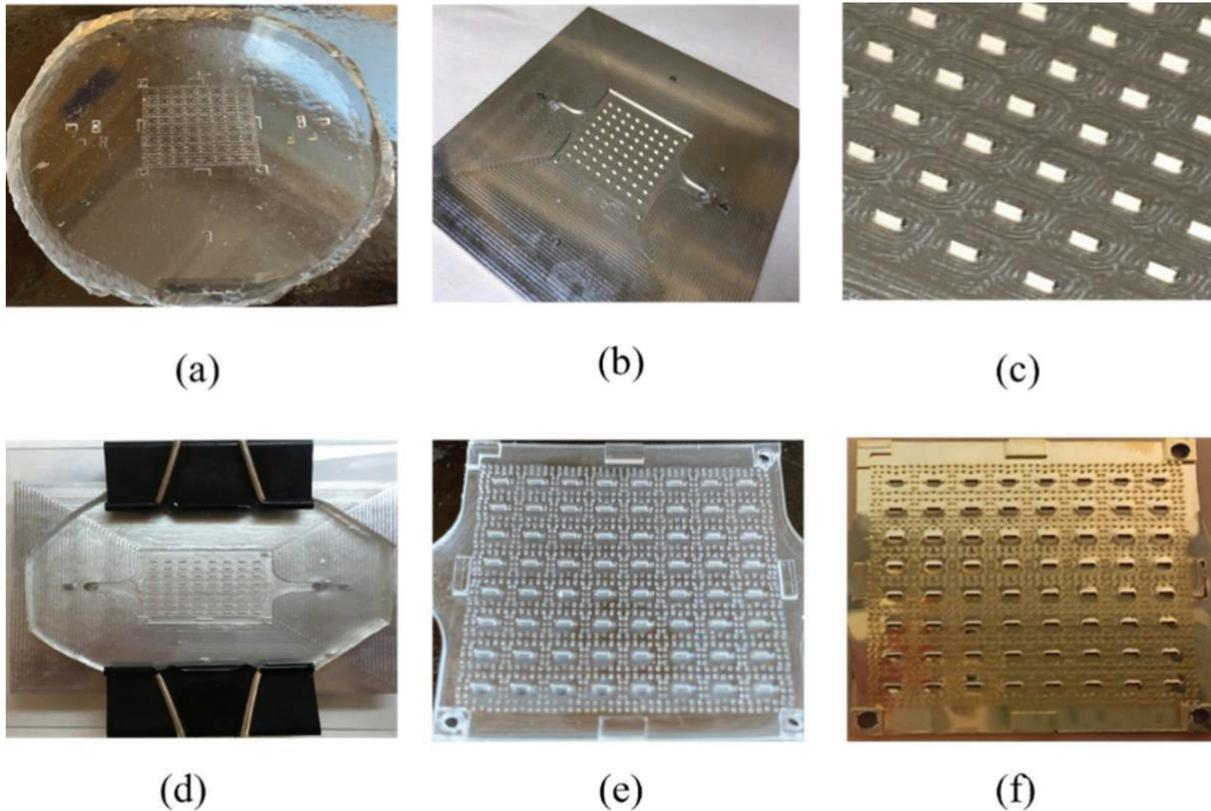
Figure 8: Injection molding steps for the cavity layer. (a) PDMS mold for the cavity layer, (b) aluminum (Al) mold, (c) closed image of the milled Al piece showing the pins to create the cavity opening after injection molding, (d) PDMS mold on top of the aluminum mold, ready for injection molding, (e) cavity layer made of OSTEMER after UV exposure and heat cure, (d) cavity layer after conductive layer deposition.
