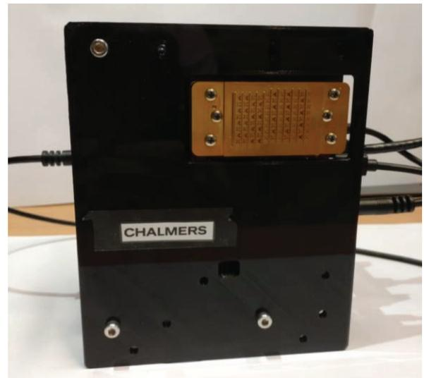
Figure 6 Demonstrator of proposed radar board.
