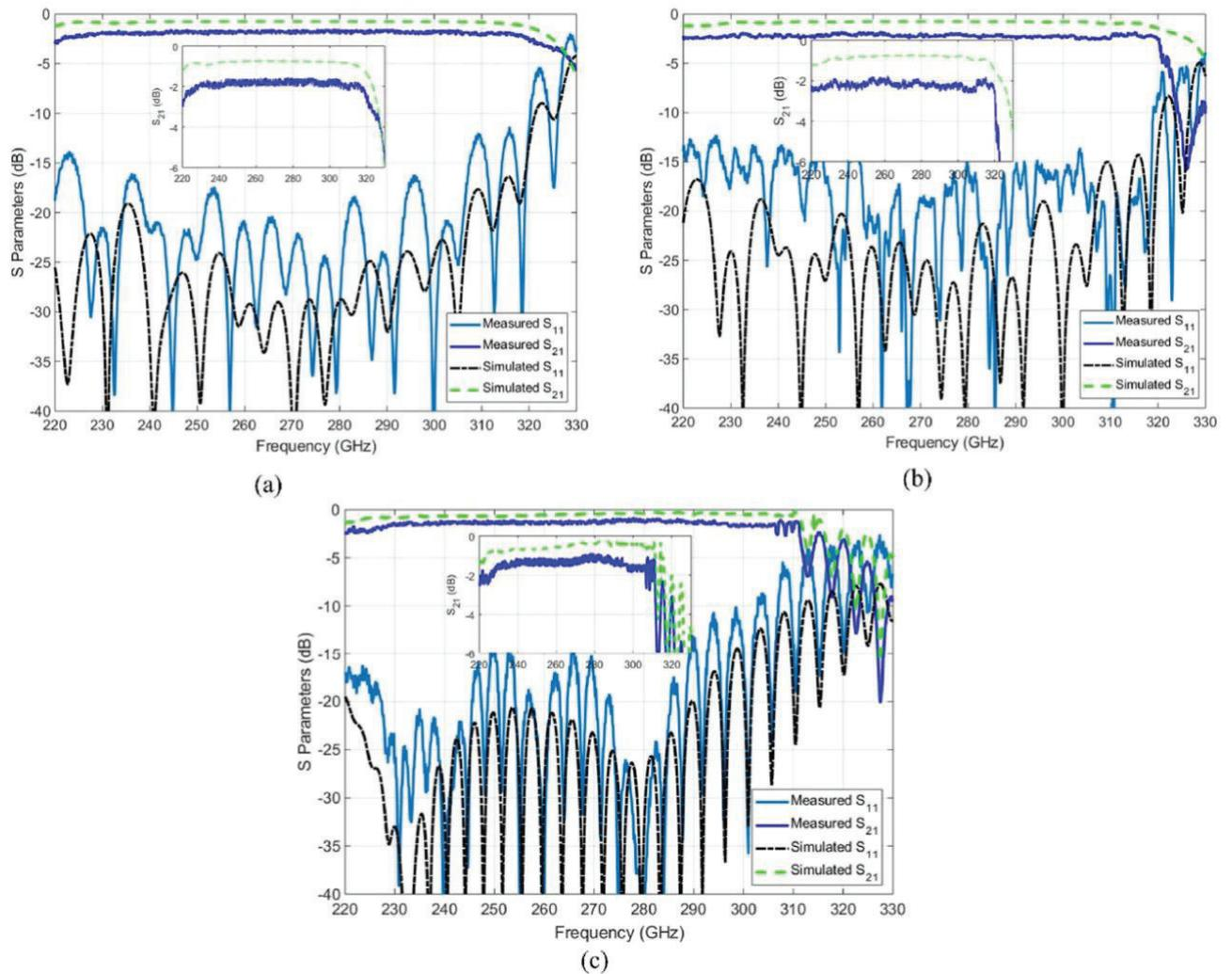
Figure 13: Measured (solid line) and simulated (dashed lines) S-parameters of the back-to-back (a) straight RGW transmission line, (b) bent RGW transmission line, (c) GGW transmission line.
