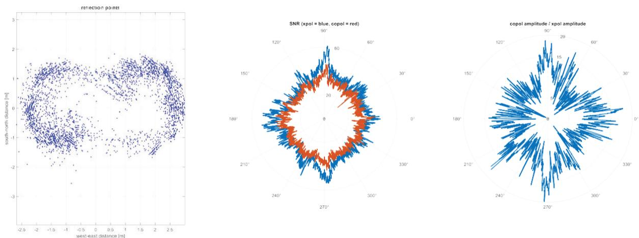
Figure 28 Data evaluation shows the detection point cloud, the SNR for both polarizations and the amplitude relationship between the two polarizations for all attitudes around the car.
