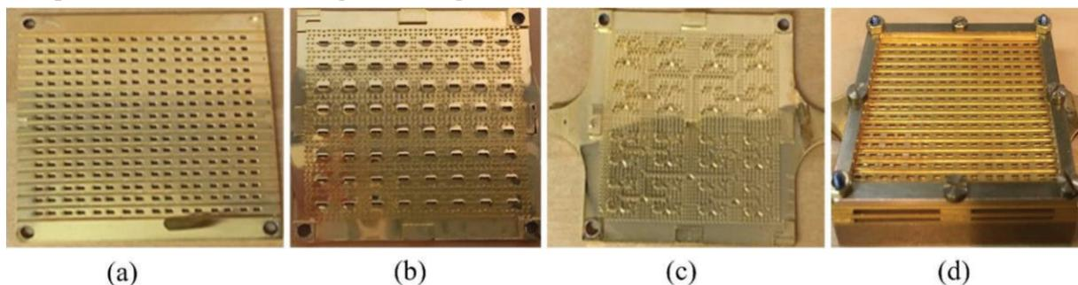
*Figure 7: Fabricated antenna, (a) slot layer, (b) feed layer, (c) cavity layer, (d) complete antenna mounted on the milled base plate.*
