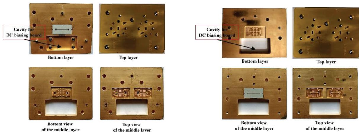
Figure 14. multi-layer display of the microstrip to gap waveguide transitions in back-to-back configuration.
