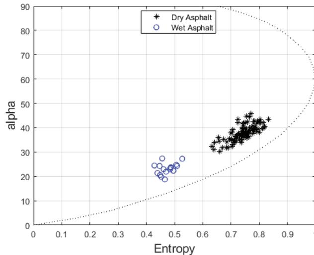
Figure 21 Asphalt of normal roughness in dry and wet condition. The dry surface is measured over a 99s interval, the wet surface patch is measured over 16s. It should be considered that  $\alpha$  and entropy are not independent. The region of possible  $\alpha$  values in the following figures is confined by the dotted lines.
