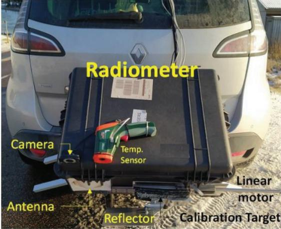
Figure 28 A picture of the radiometer mounted on a car for tests in winter conditions. The measurements were performed at the Veoneer test site at Vårgårda.
