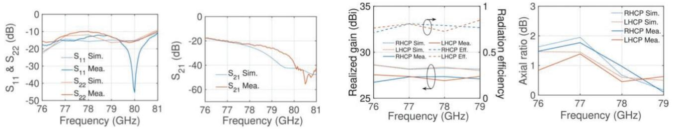
Figure 5 Measurements results of the dual circular polarized antenna 2.
