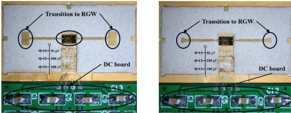
Figure 15. microstrip to gap waveguide transitions utilized in packaging of off-the-shelf MMICs.
