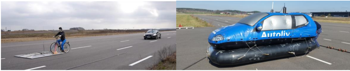
Figure 2 – A participant approaches the robot-cyclist on the airfield in Vårgårda (left). The robot-car used as oncoming traffic in the experiment (right).
