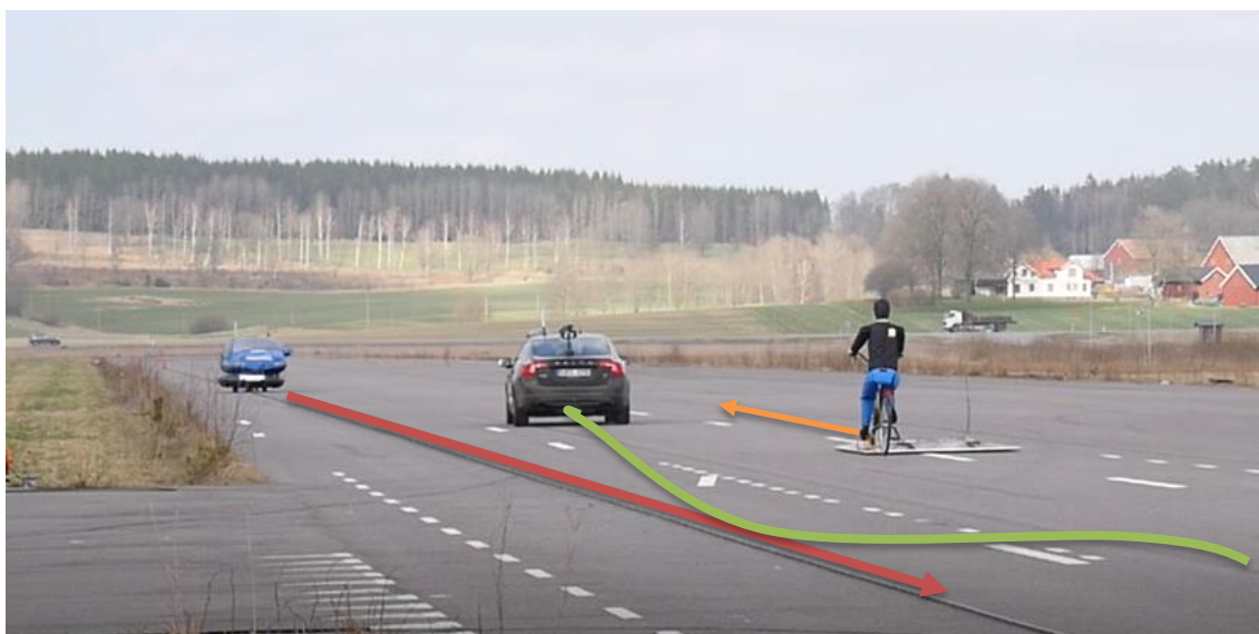
Data collection. Overtaking a robot-cyclist while meeting an on-coming robot-car at the airfield in Vårgårda.
