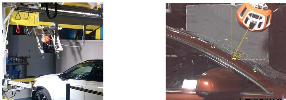
**Figure 26. Helmet-to-vehicle impact test method; overview (left), and A-pillar impact angle at 65° (right)**
