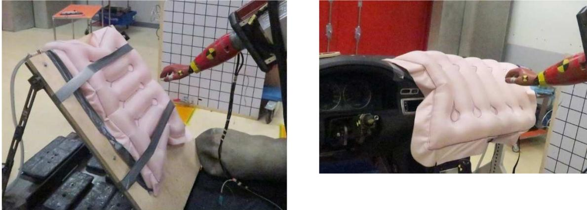
**Figure 44. Test set-ups using the novel instrumented forearm to impact the prototype ‘instrument panel airbag concept’; generic test board (left) and vehicle IP (right).**
