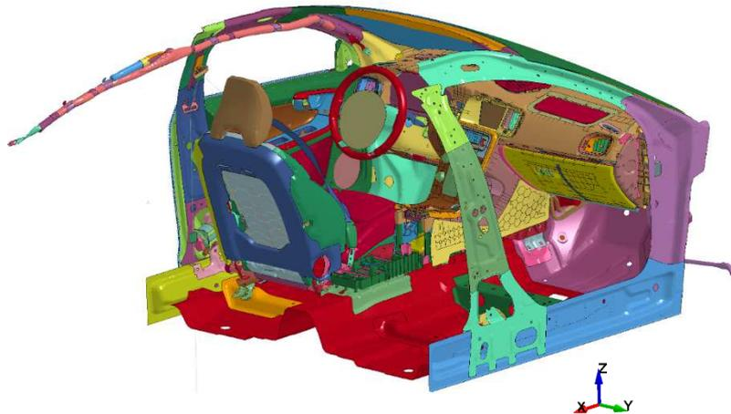
**Figure 9** The vehicle environment used in the NHTSA oblique frontal impact load case
