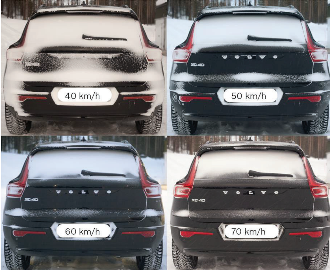
Figure 4: Snow accumulation at a rear view of an electric SUV after driving for 25 km at varying driving speeds.
