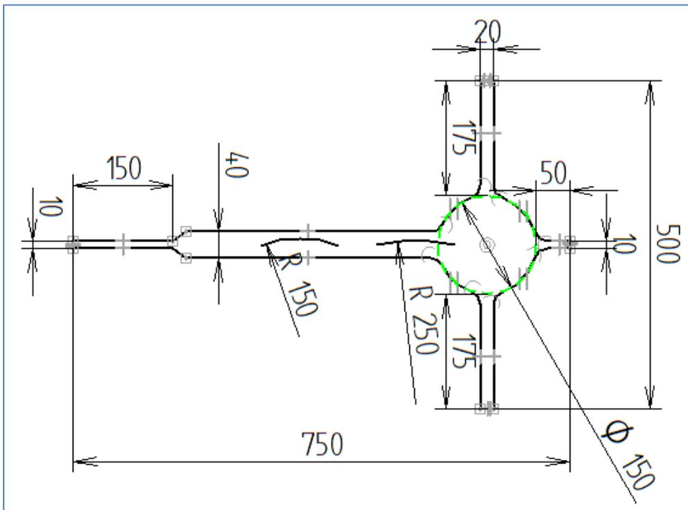
Figure 9. Example of indoor track dimension and geometry.
