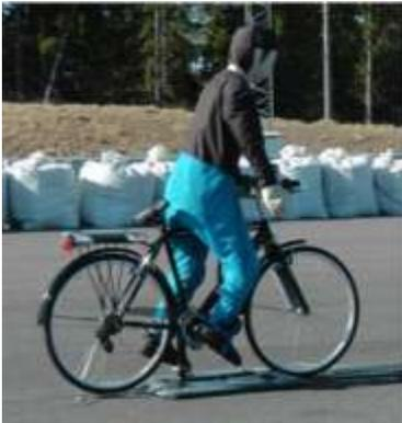
**Figure 14. Mid-speed target carrier with bicycle target mounted.**
