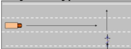
**Figure 18. Illustration of straight crossing path – bicyclist from right.**
