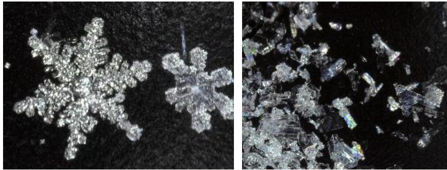
Figure 4. Snow particles a) untouched snow fresh falling b) from vehicle snow cloud
