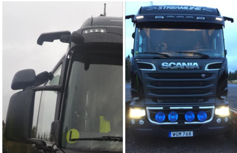
Figure 4. DREAMS camera module is mounted close to the front corners of the cabin, one on each side.
