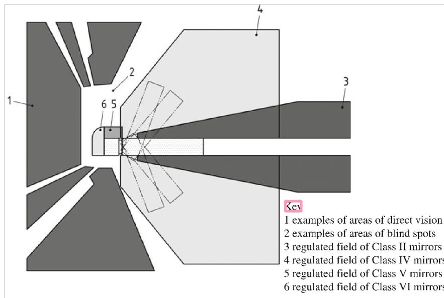
Figure 1. Different classes of mirrors on trucks as specified by UN R.46 and illustration of blind spots areas for different positions of the trailer.
