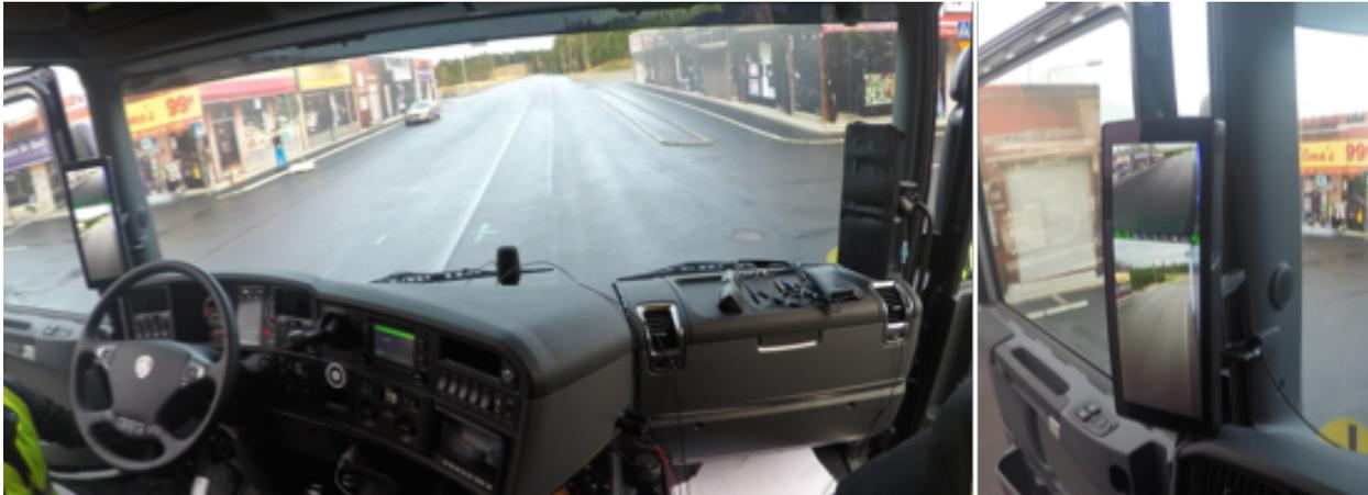
Figure 5. DREAMS monitor module is placed on the A-pillar in the track cabin, one on each side.
