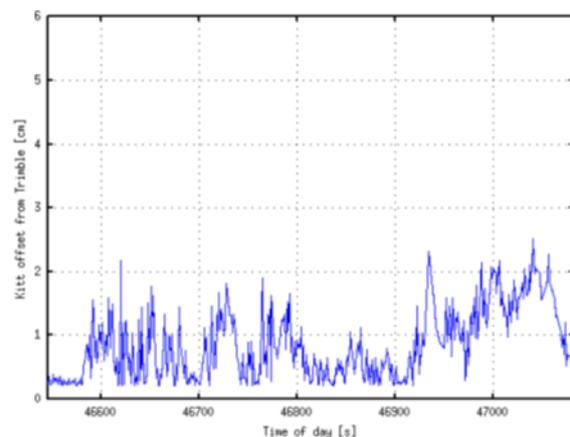
Figure 2 Measurement from the divided highway between Södertälje and Järna. The position difference in the horizontal plane between the developed system and the reference system is shown.
