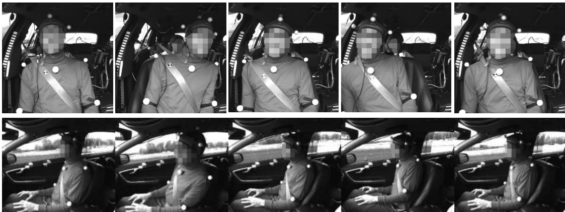
Figure 7. Video data from one male volunteer in a lane change without braking manoeuvre, front view (top row) and lateral view (bottom row) for time= 0, 0.5s, 1s, 1.5s and 2s (left to right).
