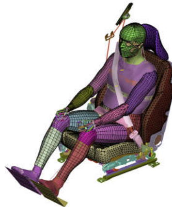
Figure 2. The SAFER HBM v9.0 positioned in the vehicle seat and restraint system for simulation of the autonomous lane-change volunteer experiments performed within the project.
