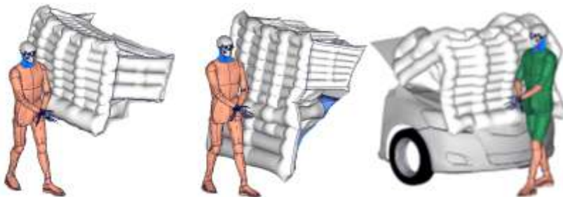
Figure 4: Three different PPA-concepts evaluated with THUMS-KTH and FEMRIPP.
