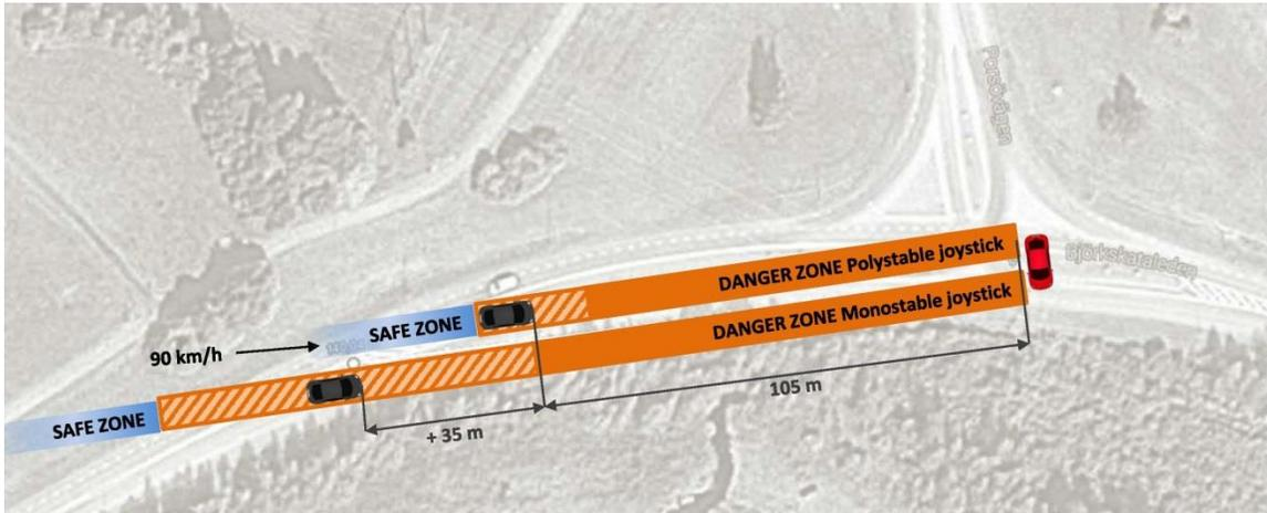
**Figure 4.** Distance needed to oncoming harm to avoid accident. The striped areas represent the variance of participant results. A monostable joystick creates a more dangerous situation than a polystable joystick.
