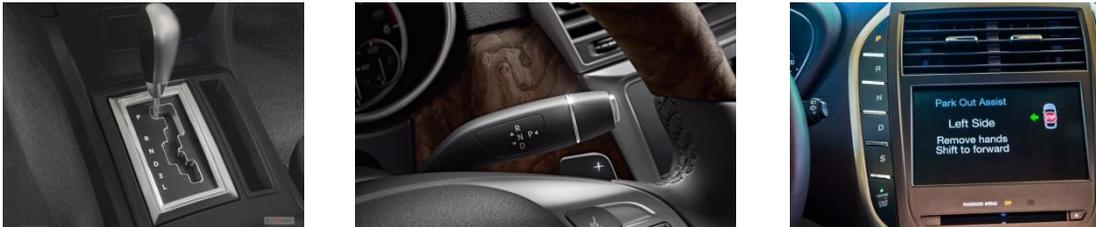
**Figure 1.** A traditional worm gate joystick, a Mercedes ML350 stalk shifter and a Lincoln MCS button shifter.
