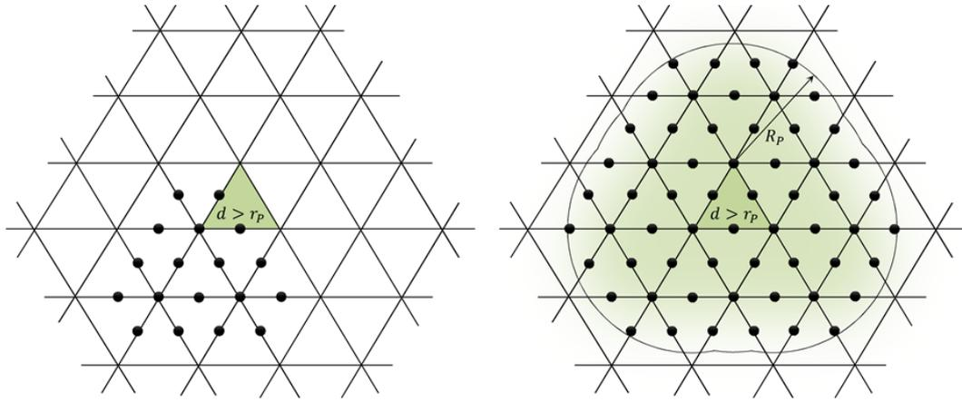
Figure 10. When damage is initiated in a cohesive law (left), the delamination enrichment patch (marked by •) is expanded to include all nodes within a radius  $R_p$ . From [3].
