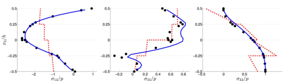
Figure 11. Transverse stress components in reference 3D (blue solid) and shell (red dashed) models together with recovered stresses ( $\bullet$ ) at  $\mathbf{x}_3 = L/3$  in simply supported beam. From [3].
