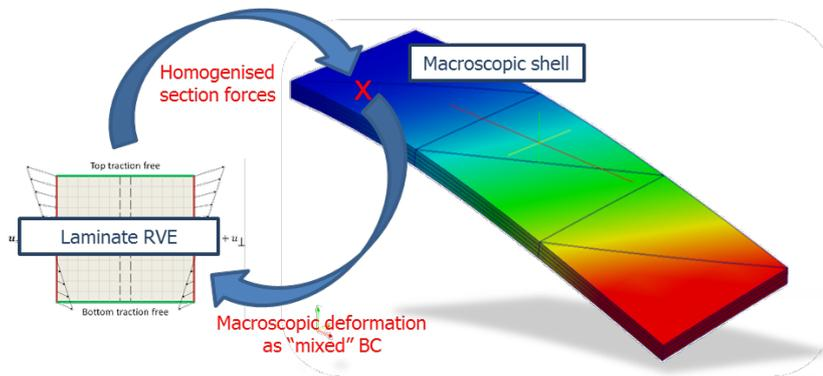
Figure 1. Generic sketch of a multi-scale approach where the material behaviour is analysed on the meso-scale level via a detailed RVE analysis to predict damage evolution in individual plies given the macroscopic deformation as boundary conditions. The resulting homogenised section forces of the shell are then transferred back from the RVE to the macroscale level and used as input to solve for the component deformations.
