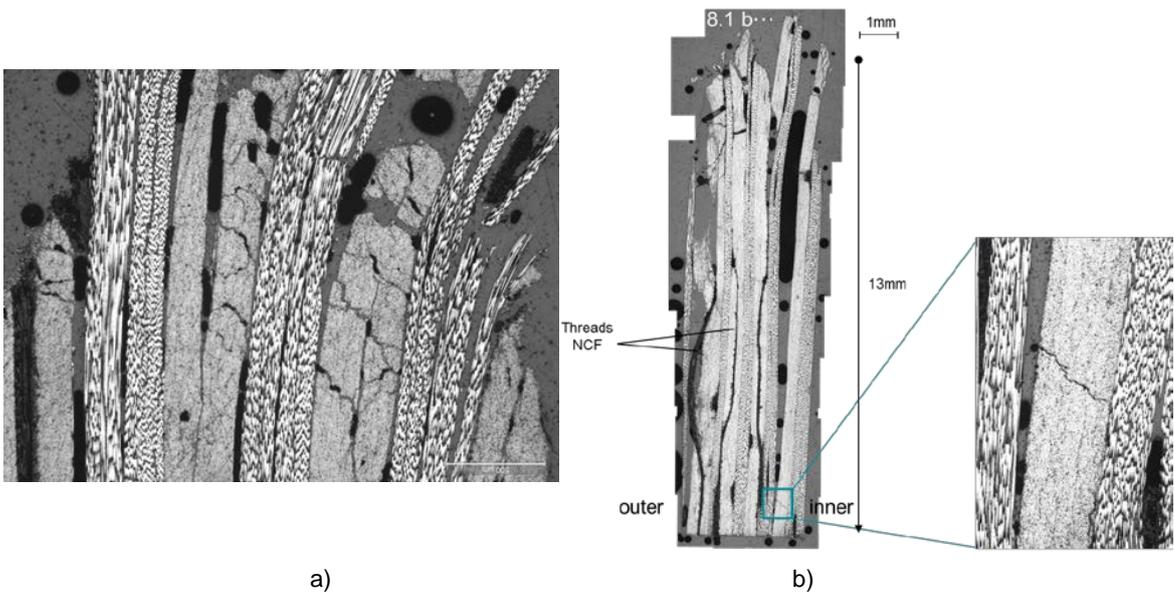
Figure 31. Delaminations and intralaminar failure observed from the microscopic studies of the crash boxes
