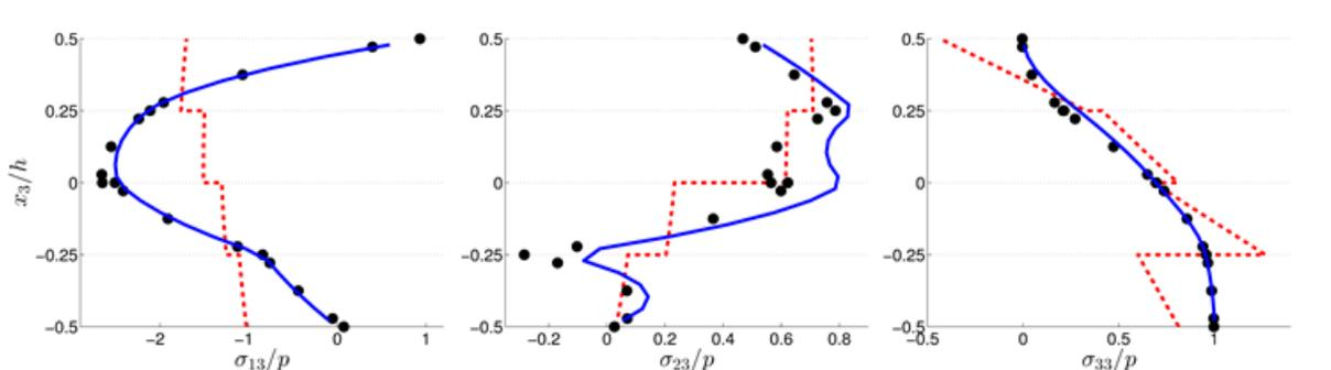
Figure 11. Transverse stress components in reference 3D (blue solid) and shell (red dashed) models together with recovered stresses ( $\bullet$ ) at  $x_3 = L/3$  in simply supported beam. From [3].
