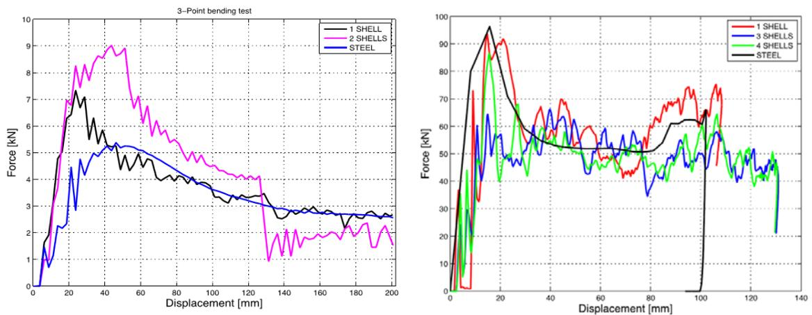
Figure 20. Analysis results of door beam bending load case (left) and crash box crushing (right) for both a steel and a composite design
