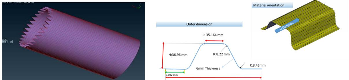
Figure 14. Prototype design of the crash box component (left) and the beam component (right).
