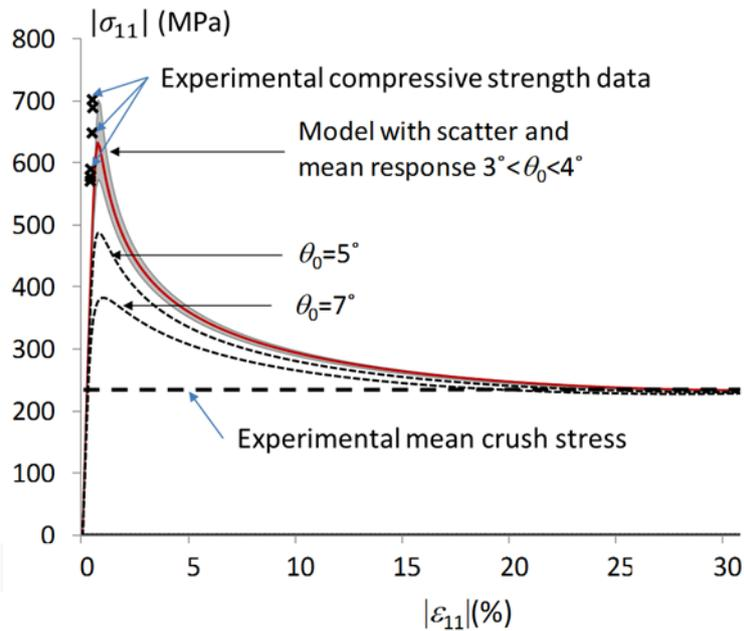
Figure 9. Prediction of compressive behavior and comparison with experiments for different fiber misalignment angles  $\theta$
