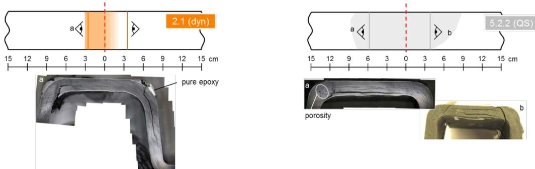
Figure 21 Results from A-scan of two of the tested beams
