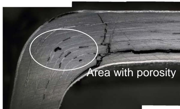
Figure 30. Image on existing porosity at the beam shoulders resulting from the manufacturing
