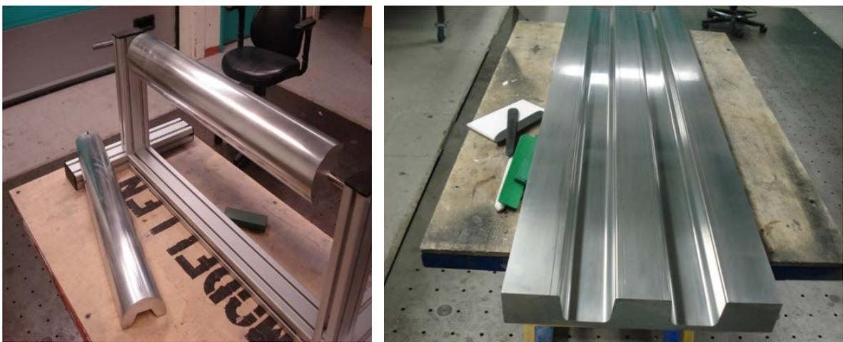
Figure 3. The aluminium tools for the crash box (left) and for the beam (right).
