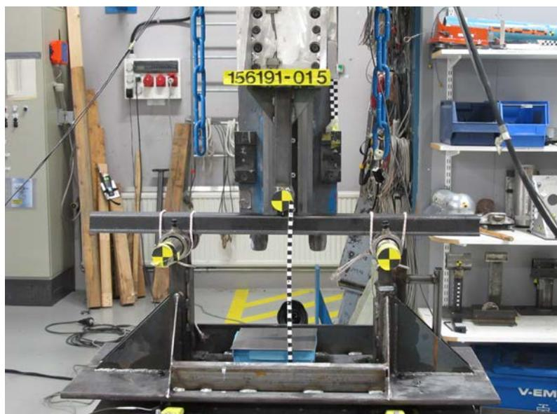
Figure 5. Drop tower rig used for dynamic beam testing
