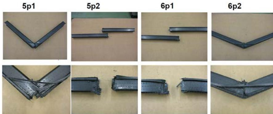
Figure 17. Beams after quasi-static testing
