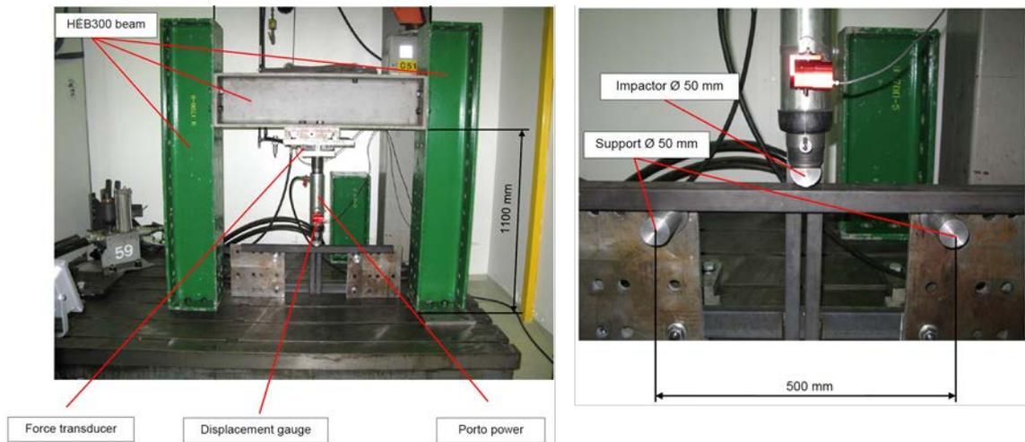
Figure 4. Rig used for quasi-static testing
