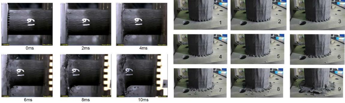
Figure 21 Dynamic crushing left and quasi-static crushing right
