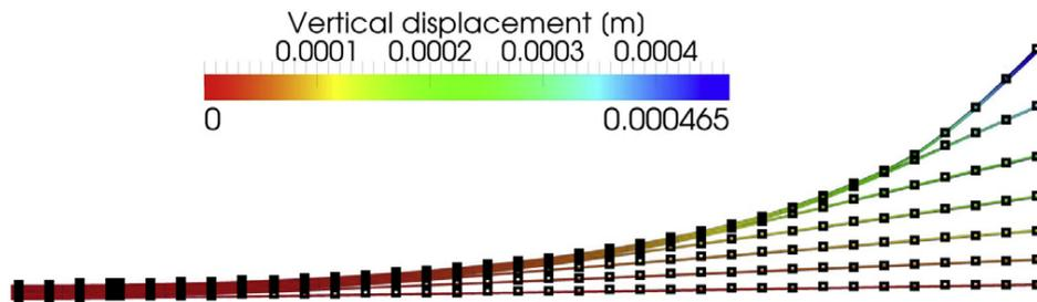
Figure 2. Illustration of the ability of the adopted XFEM shell concept to represent multiple (six) delamination cracks of different length using only one shell element through the thickness. The FE result is in the figure compared with the analytical solution to the problem (black squares).
