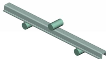
Figure 7. The model of the three-point bend test used in the master thesis carried out at Semcon
