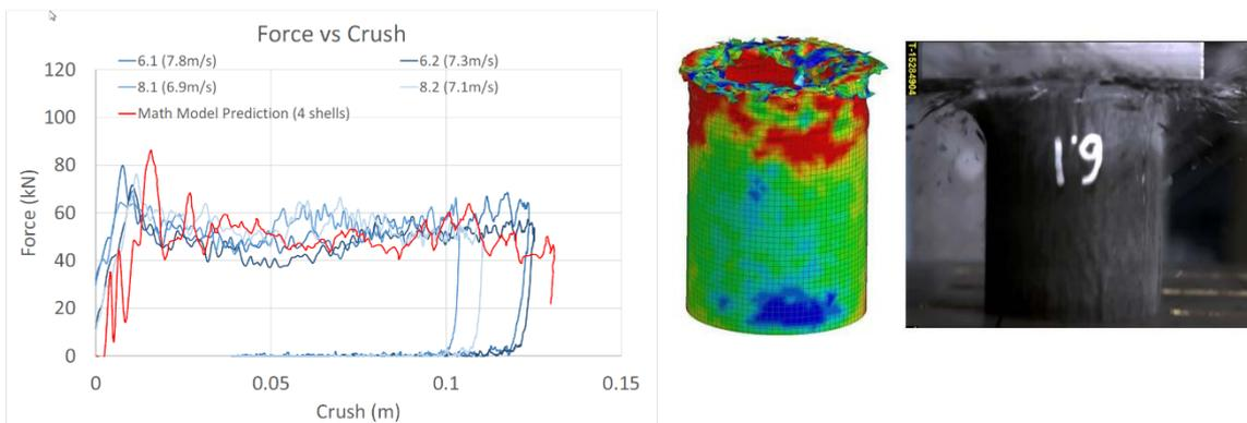
Figure 24. Dynamic tests compared to simulation
