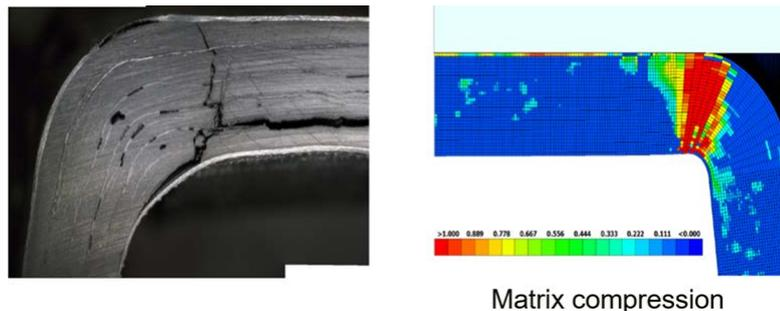
Figure 22 Comparison between experiment (fractography to the right) and modelling results (with SICOMPs material model to the left)
