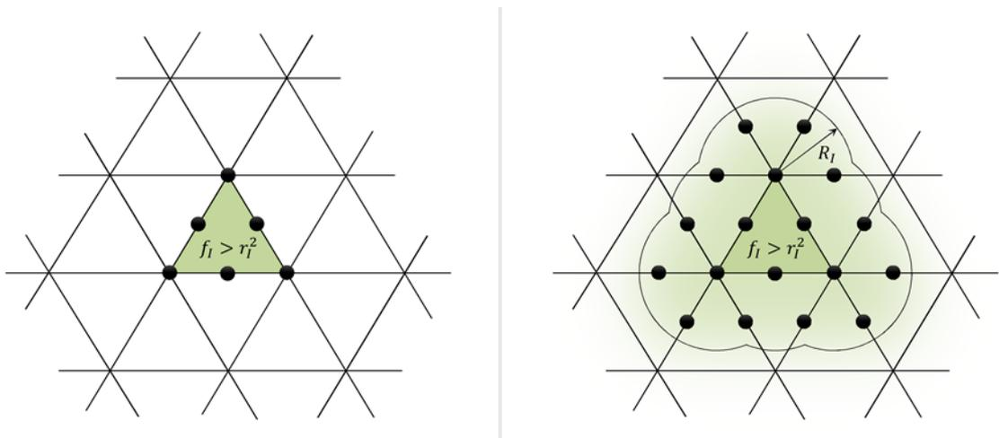
Figure 9. When the initiation criterion  $f_I$  exceeds the threshold value  $r_I$  in an element the associated element nodes are enriched (left) along with the nodes within a radius  $R_I$  (right). From [e].
