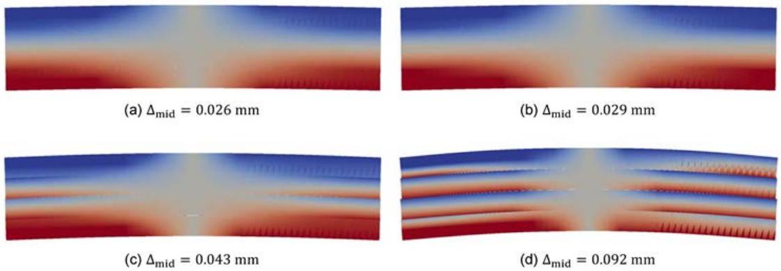
Figure 16. Deformation plots of the adaptively enriched simply supported beam: (a) after delamination enrichment initiation but prior to expansion, (b) after delamination propagation in mid interface, (c) after all delamination enrichments have been initiated, expanded and all delaminations has started to propagate and (d) final deformation before top interface detaches. Five times deformation scale. From [3].
