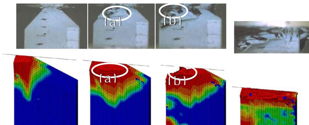
Figure 8. Experiments and model prediction during crushing transverse to fibres.
