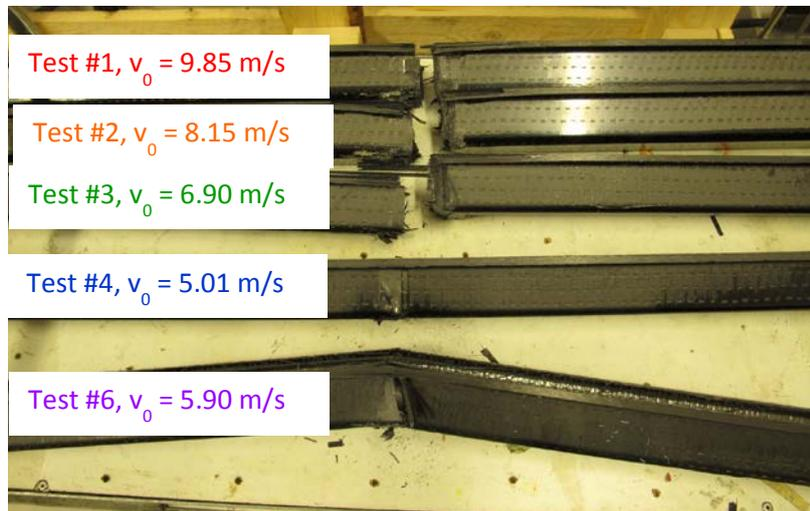
Figure 19. Dynamically tested beams
