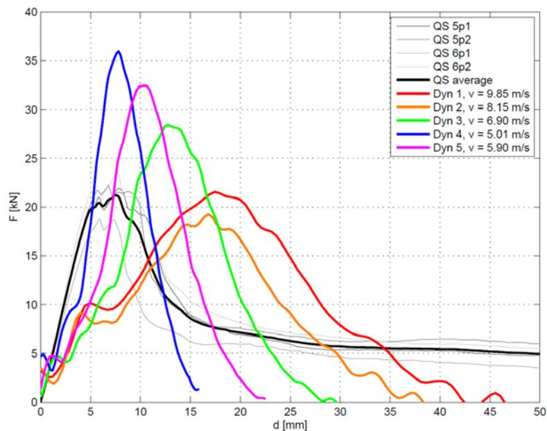
Figure 20. Force displacement curves from quasi-static and dynamic beam tests
