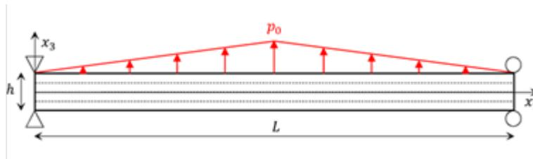
Figure 11. Simply supported  $[0]_4$  beam used to exemplify the adaptive delamination modelling methodology. A vertical traction load is applied on the top surface. The beam has a low thickness to length ratio which will lead to delaminations being initiated in the mid interface at the supports of the beam. From [3].
