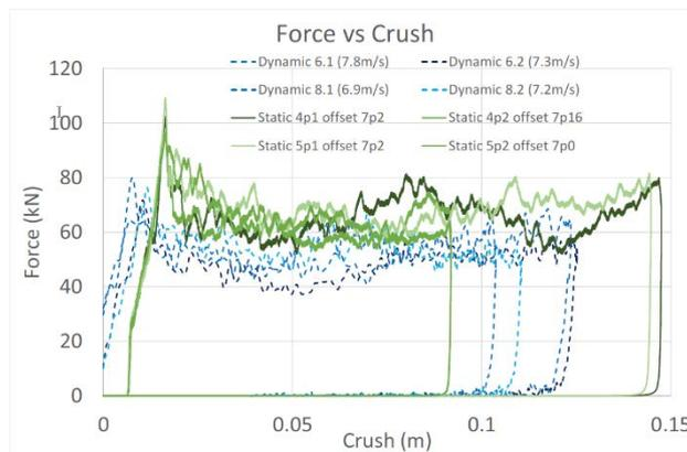
Figure 163 Crushing force crash boxes
