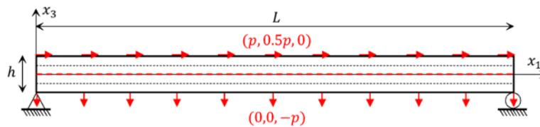
Figure 10. Simply supported [90/-45/45/0] beam used to illustrate the stress recovery technique. A negative vertical traction  $p$  is applied to the bottom surface and on the top surface shear tractions  $p$  and  $0.5p$  are applied in the  $x_1$  and  $x_2$  directions respectively. The red dashed line indicates a cohesive interface. From [3].
