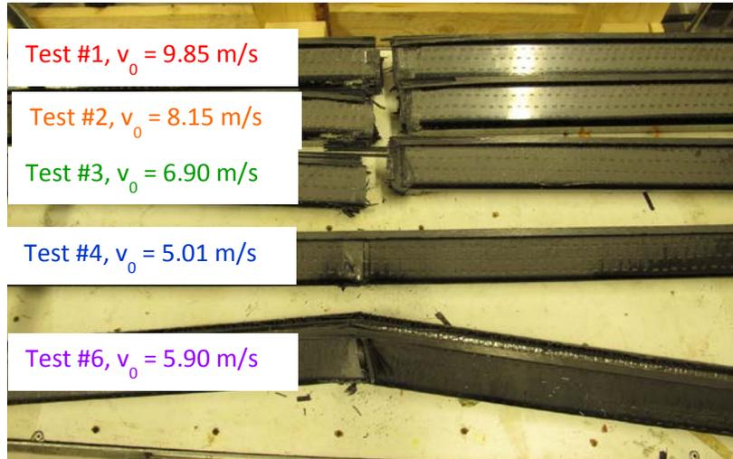
Figure 19. Dynamically tested beams
