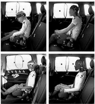
Figure 5. Maximum forward displacement of child volunteers (top), Q6 (bottom left) and HIII 10y (bottom right) kinematics in evasive braking maneuver of 1g.
