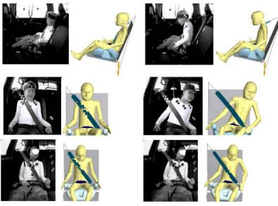
Figure 6. The active child HBM compared to volunteers at start and at maximum head displacement for a braking event (top row), a 0.8g steering event (middle row), and a 0.6g steering event (bottom row), (Brolin et al. 2015)
