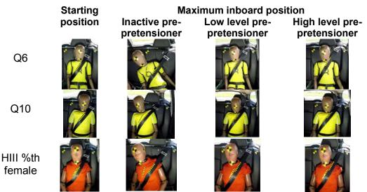
Figure 8. Q6 (top row), Q10 (middle row) and HIII 5th female (bottom row) in starting position (left column), and maximum inboard position for the three prepretensioner settings (Bohman et al. 2016)
