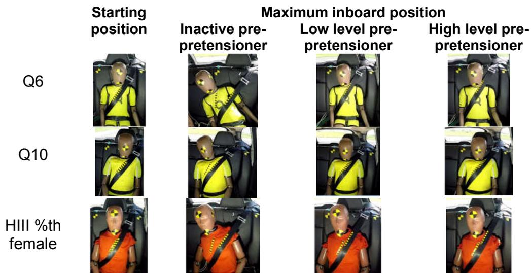
Figure 8. Q6 (top row), Q10 (middle row) and HIII 5<sup>th</sup> female (bottom row) in starting position (left column), and maximum inboard position for the three pre-pretensioner settings (Bohman et al. 2016)
