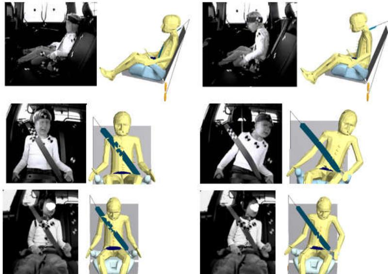
*Figure 6. The active child HBM compared to volunteers at start and at maximum head displacement for a braking event (top row), a 0.8g steering event (middle row), and a 0.6g steering event (bottom row), (Brolin et al. 2015)*
