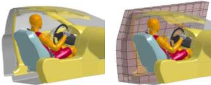
**Figure 1.** The updated generic side impact FE model, including the Autoliv THUMS human FE model (left) and the same model but with the coarse grid boundary condition (right) overlaid.
