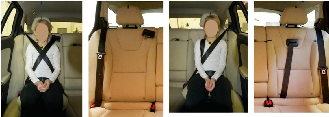
**Figure 1** Two belt geometry concepts – adding a 2-point belt to the conventional 3-point belt.
