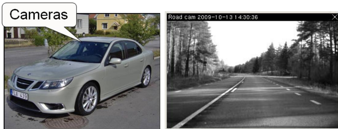
Figure 3. Location of- and output from one of the forward looking cameras.
