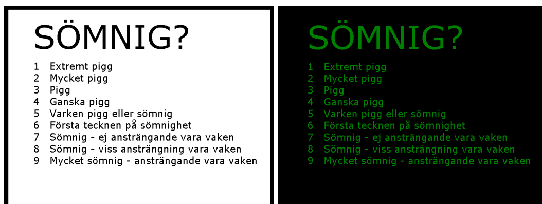
Figure 7. The screen prompting the driver to report KSS (Karolinska Sleepiness Score). Daytime and nighttime appearance.
