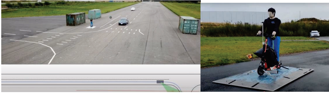
Figure 6: Left: experiment setup showing the right-turn intersection including both the dummy e-scooter rider and the ego vehicle. Right: close-up of the e-scooter dummy target on the remote-controlled platform.
