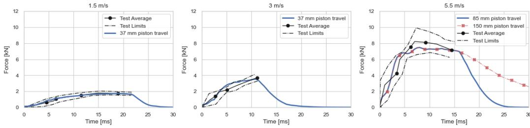
Figure 15. SAFER HBM v11 responses to Forman et al. (2015) back hub impacts with the HBM response in blue and red, compared with the experimental data in black. Figure extracted from the Jupyter Notebook Validation Catalogue developed in the project.
