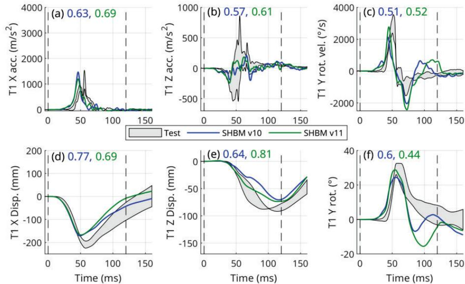
Figure 18. HBM T1 kinematics in the upright (25°) position in comparison with PMHS data from Kang et al. (2020). The number after the letter notation for each panel is the ISO score, and the time interval used for its calculation is indicated by the dashed lines. Acc. = Acceleration; Disp. = Displacement; Rot. = Rotation; Rot. Vel. = Rotational Velocity. Figure adapted from Östh et al. (2024).
