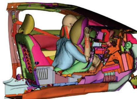
Figure 6. The interior model and the SAFER HBM v11.0.1 in the accident reconstruction.
