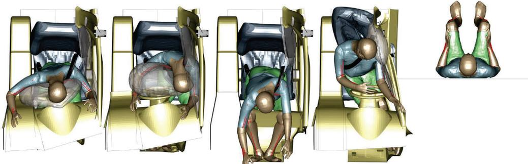
Figure 4. SAFER HBM high severity robustness verification load cases. From left to right: driver frontal impact, driver oblique impact, rear seat frontal impact, driver side impact and free fall on the back to rigid surface.
