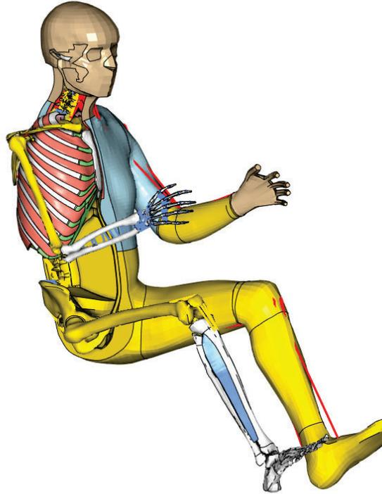
*Figure 14. The resulting SAFER HBM v11 after updating. The gold/yellow body parts are parts which have been updated or replaced since the previous model version within this project.*
