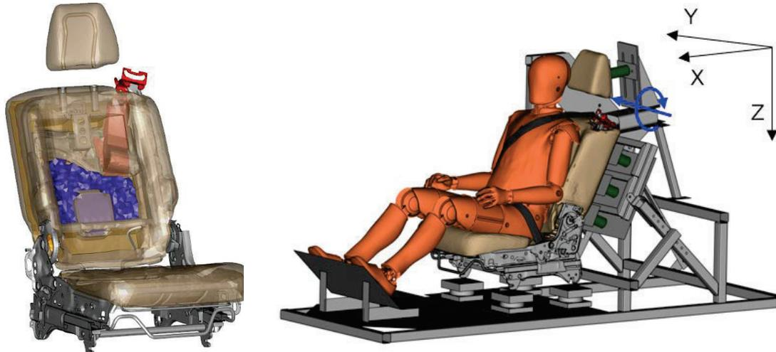
Figure 7. Seat model (left) and sled model with the THOR crash test dummy (right) developed for high-speed rear facing frontal impact validation of the SAFER HBM and comparison to the crash test dummies THOR, Hybrid III and BioRID. Figure adapted from Östh et al. (2024).
