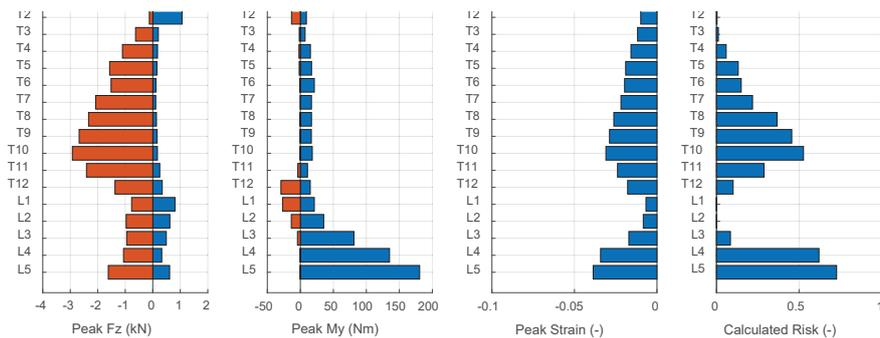
Figure 16. Peak vertebral cross-sectional  $F_z$  force and  $M_y$  moment, and peak superior-inferior strain and associated lumbar vertebra body fracture risk for the accident reconstruction simulation.
