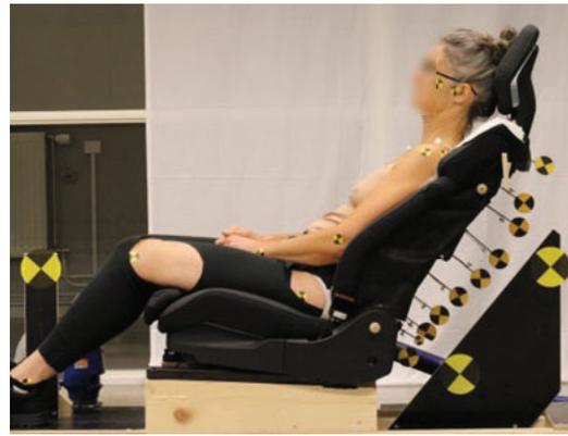
*Figure 2. Volunteer seated in the reclined seating posture with film marker instrumentation.*
