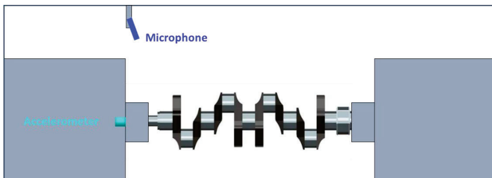
Fig. 24. A schematic representation of the accelerometer and microphone placement within the Scania crankshaft production line
