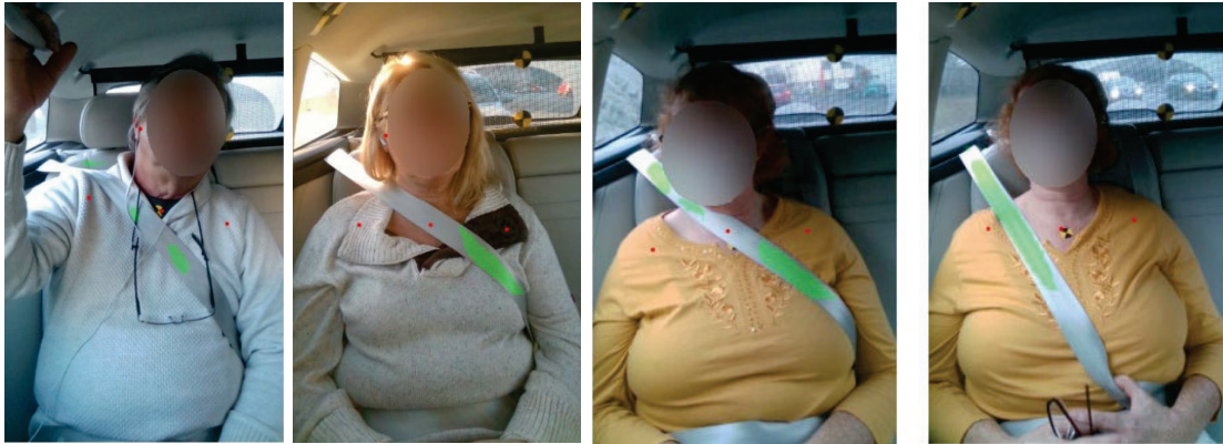
Fig. 9. Example of how test persons' body shape influence beltfit and chosen strategies (right) to reposition the shoulder belt during the ride (Makris et al., 2023)
