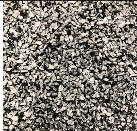
Figure 31 "dust separated" by milling twice
