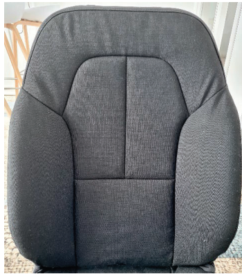
Figure 7. Seat appearance with a one-polymer solution of polyester.
