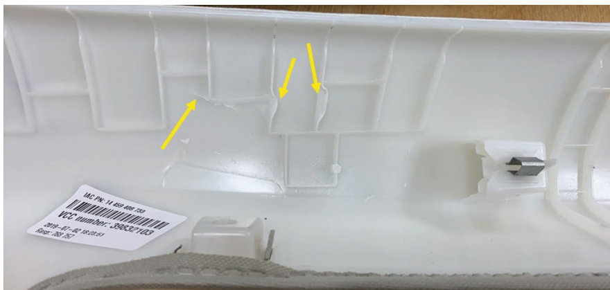
Figure 35. Pillar with 100% virgin content . Arrows showing deformation and crack from crash test
