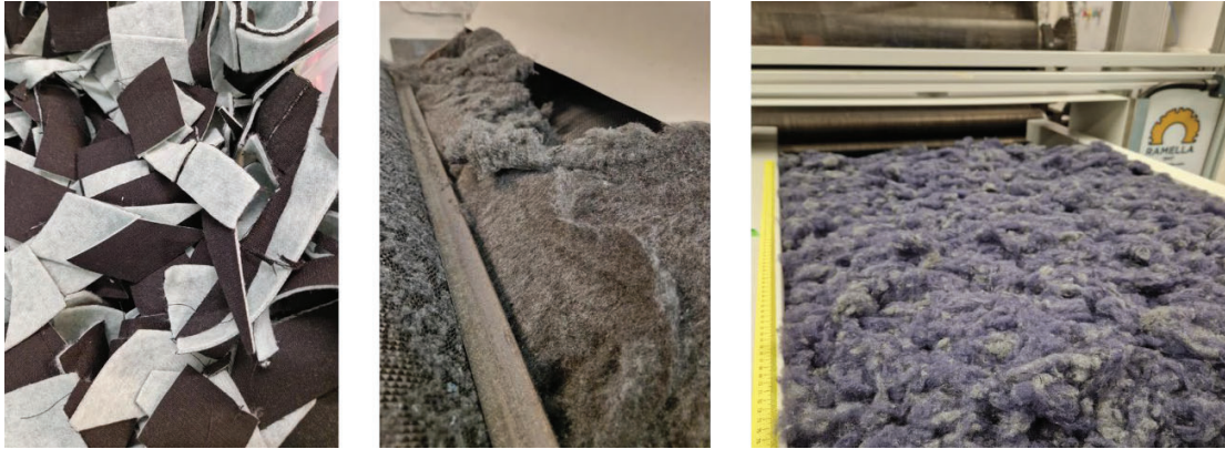
Figure 8. Cut one-polymer solution upholstery to the left, material during shredding in the middle and fibers going into the carding machine to the right.
