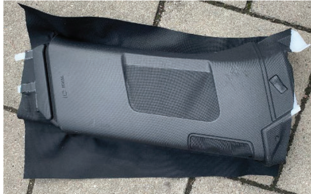
Figure 5. Textile covered pillar made of PC/ABS with polyester textile covering
