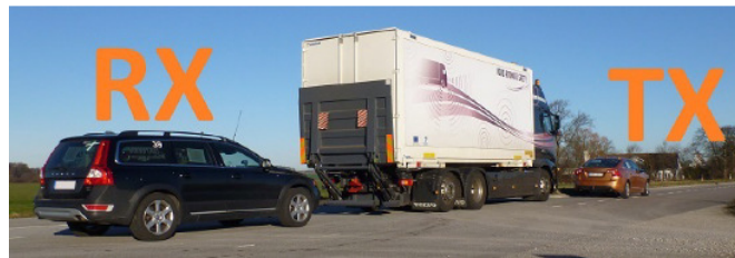
Figure 12. Characterization of the influence of trucks and larger objects on the V2V link between the Tx and Rx cars. The Tx car is here equipped with 6 antennas at various positions.
